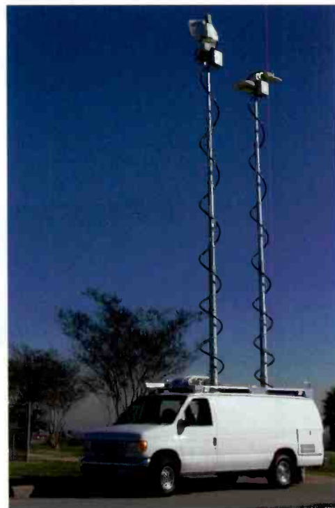
The E-N-G Mobile Systems EasyLINK II HDTV microwave news van is equipped to operate with NTSC, SDI and HD inputs.
