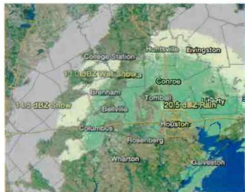
The image shown here is hydrometeor classification from dual-polarization radar. Image courtesy Baron Services.
