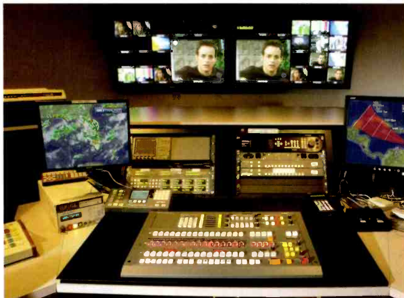
WINK's on-air master control center features a Grass Valley master control switcher and two 50in Panasonic HD plasma monitors fed by a Miranda Kaleido-K2 dual-head monitor wall processor.
