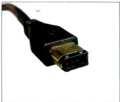
An IEEE 1394 (aka FireWire or i.Link) cable offers a bidirectional connection terminated in a six-pin connector (shown here) or in a smaller four-pin.
