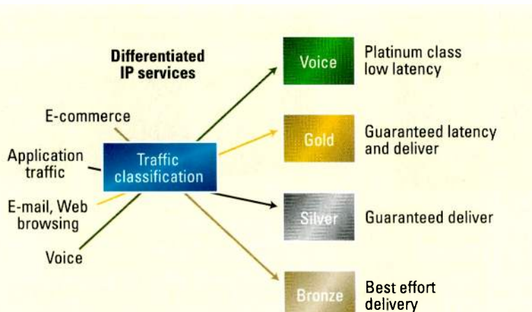
Figure 2. In the Differentiated Services protocol, packets from various applications are classified as they enter the network.
