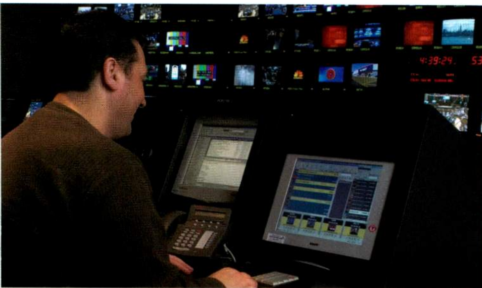
At CNBC, a Grass Valley NewsBrowse Web-based browser/editor manages a file-based news system.
