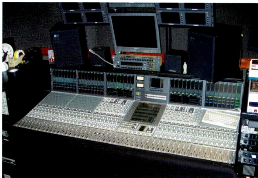
SSL's C100 digital audio console allows audio mixers with Studio 58 to program each fader to function as an individual channel input, a stereo input or a 5.1 mix fader.
