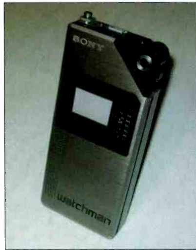
Mobile TV isn't new. In 1982, the Sony Watchman allowed consumers to watch NTSC broadcasts virtually anywhere.
