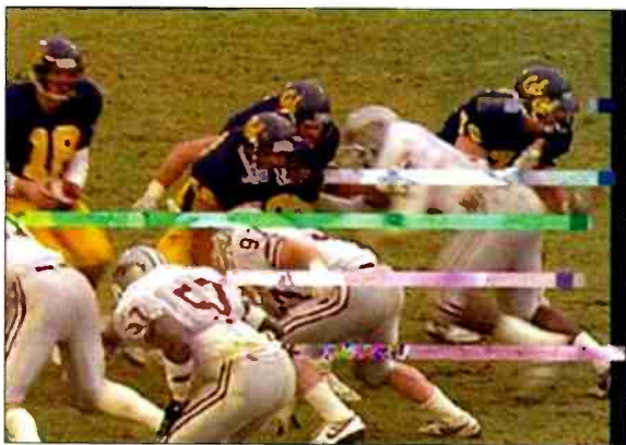
Photo 1. An illustration of what the customer sees. In this example, the picture's I-frames are missing.
