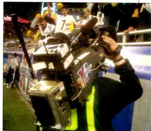
At the 2006 Super Bowl, ABC used Grass Valley LDK 6000 HD cameras equipped with Link Research LinkHD COFDM transmitters, as supplied by Aerial Video Systems.
