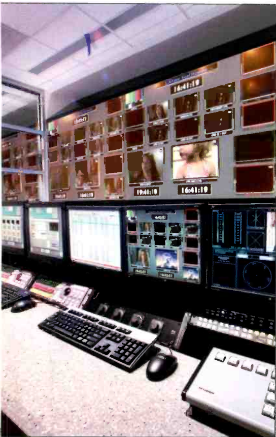
This master control pod is used for playback and monitoring of Lifetime Movie Network and Lifetime Real Women.
