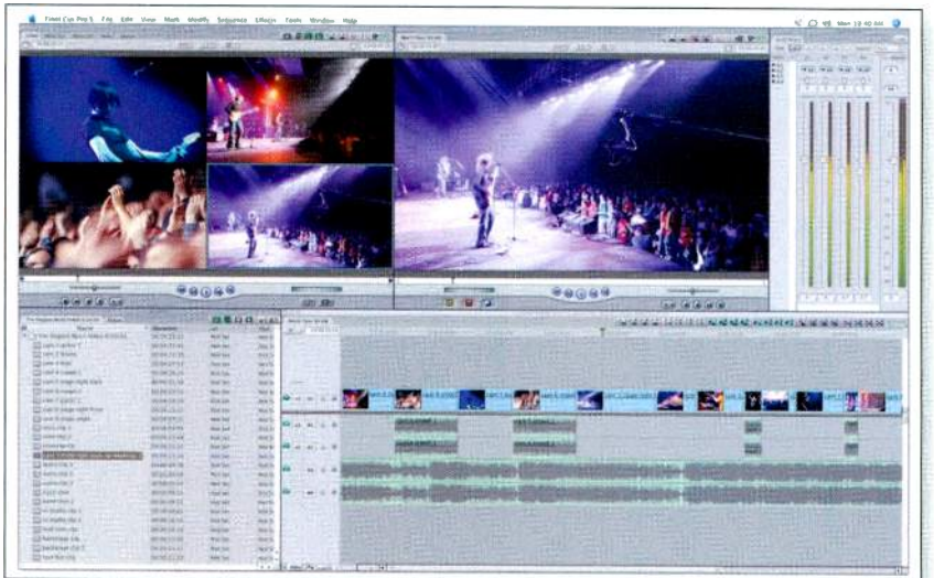
Apple's Final Cut Pro acquires HDV media via FireWire and keeps it in the original format, transferring it into the system without any generation loss.
