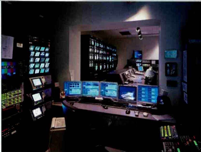
The tape/server operations room looks into the production room. It uses Sony Digital Betacam, a Grass Valley M-Series iVDR, and DNF and Lance controllers.
