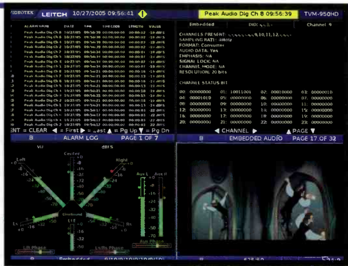
Figure 4. TVM-950HD multi-pane display including audio alarm log and level alert message
