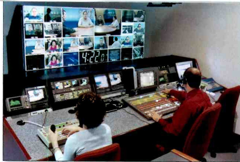
In studio control, the director/TD operates the Grass Valley Zodiak with a Chyron Duet and Panasonic remote camera control unit on either side. Behind the console is the audio booth and a producer's station, which includes the call screener and teleprompter crew positions.
