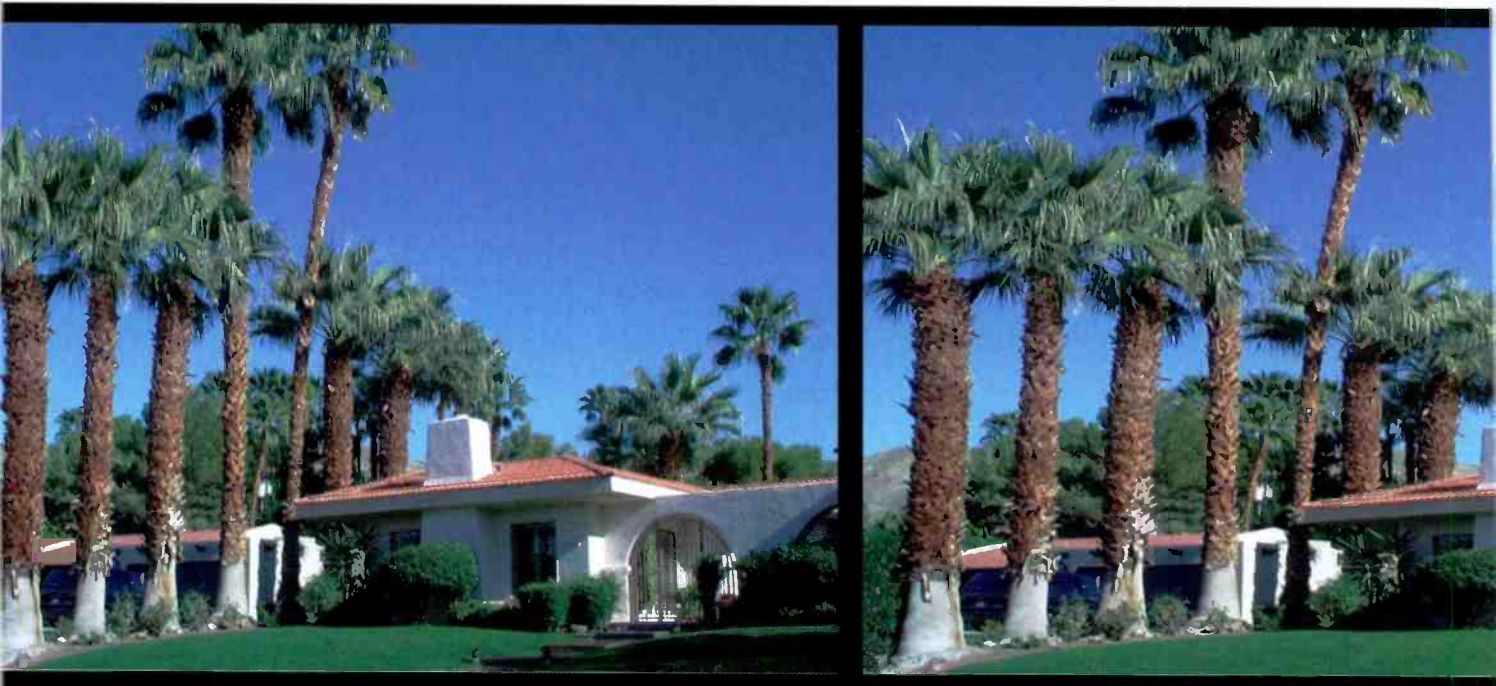
Figure 2. The figure at right is an obvious distortion of shape and elements that occurs when a graphic originally created for 4:3 (shown at left) is stretched to fit a 16:9 display.
