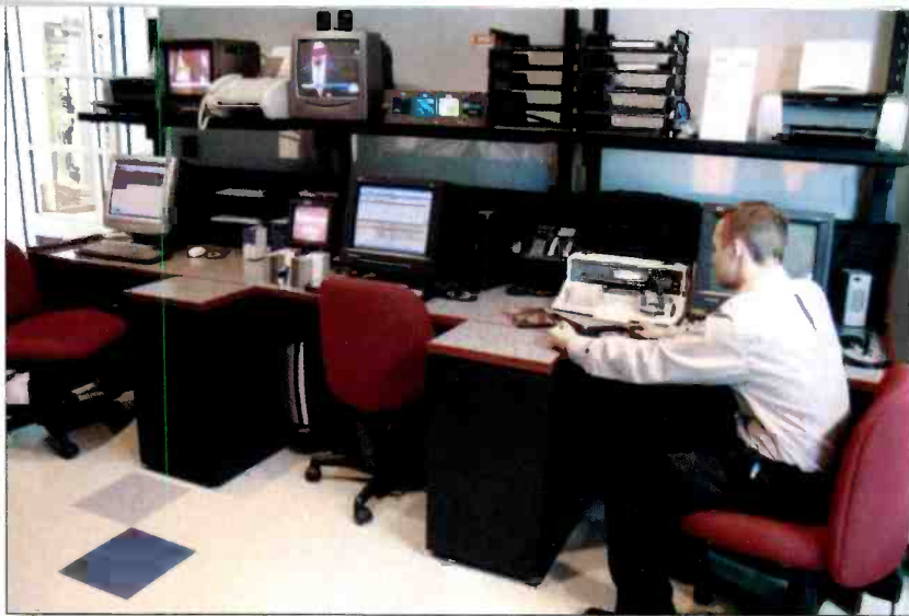
Three workstations provide areas for Leightronix automation, Leitch video server programming and a networked PC that serves several purposes — a Chyron typing location, VHS tape labeling and a Primera Bravo DVD duplicator, which serves as a backup to the two Rimage systems.
