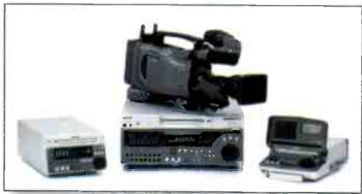
With Sony's XDCAM HD, users can record 1080i video at three data recording rates: 18Mb/s, 25Mb/s and 35Mb/s.
