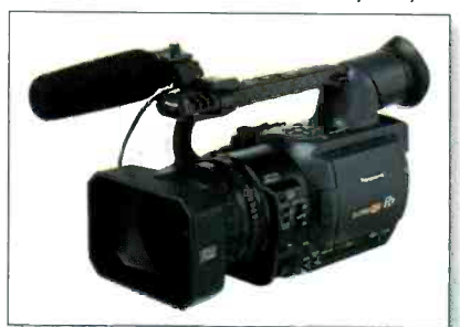
Panasonic's AG-HVX200 DVCPRO HD P2 handheld camcorder provides 1080i and 720p recording with 100Mb/s DVCPRO HD quality.
