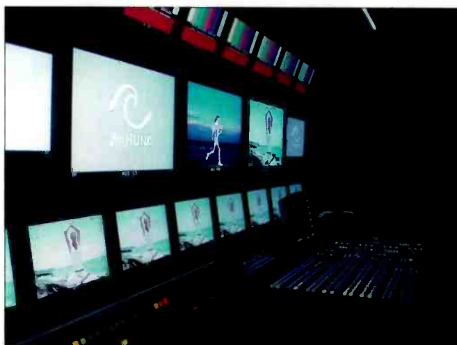
The UK's Neon Broadcast Services employs an SD/HD Kahuna production switcher from Snell & Wilcox in its newest mobile truck.
