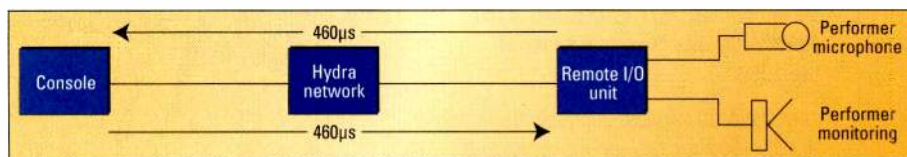
Figure 3. Low network latency is crucial when a performer is listening to a mix that includes his own voice because the signal makes two trips across the network as part of a foldback mix. The total delay is less than 1ms.
