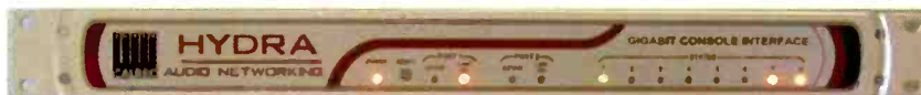
Photo 1. The front panel of the Hydra interface box, which interfaces the mixing console to the network.
