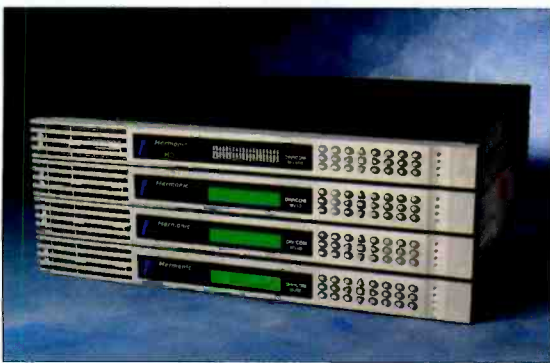
Harmonic's encoders can package MPEG video into an IP-based stream.
