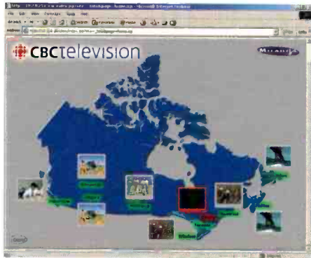
Figure 2. The main status page of the CBC's centralized monitoring of remote operations features a national map with alarm and off-air video display capability streamed back from each location via a TCP-IP network.
