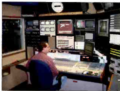
Henry Brown, Senior Audio Operator at CanWest Global, works at the facility's new Wheatstone TV-80 console.
