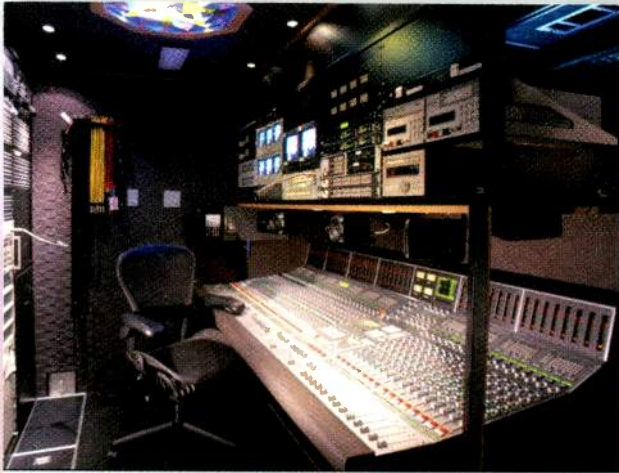
Turner Studios' 53-foot production truck, Mobile Unit #TS1, uses Solid State Logic's Aysis Air Plus console.
