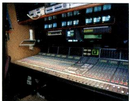
Core Digital Technologies/SWTV's expandable Sundance truck sports a 96-channel SSL Aysis Air Mobile digital broadcast console.
