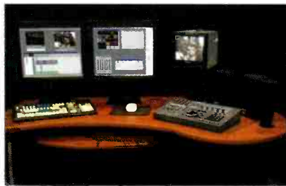
The Leitch NEWSFlash-II nonlinear editor can edit multiple compression formats and render the output to the compression format of choice.
