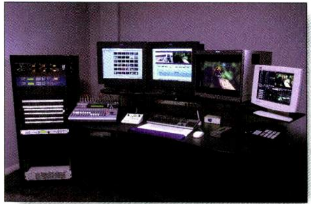
The Avid|DS HD suite is used to edit, mix and create high-definition programming at the Discovery Communications' technical center in Bethesda, MD. Photo by John Spaulding, Discovery Communications.
