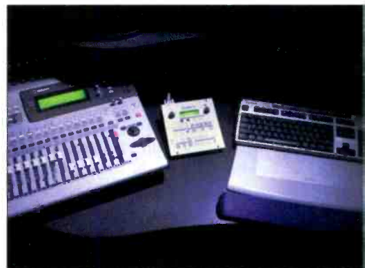
AES audio passes between the patchbays and the Avid via a Yamaha 01V mixer. A MartinSound MultiMAX was added to the suite to give editors a wide range of monitoring options. Photo by John Spaulding, Discovery Communications.
