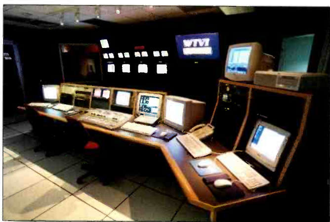
The master control is built around a Philips (now Thomson) Saturn master control system and routing, and is designed to be run as a one-man operation.
