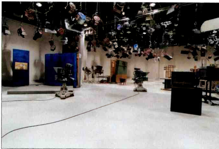
The studio equipment consists of four Philips LDK 6000 1080i cameras, ARRI lighting and QTV prompting, which is fully computerized and controlled from the control room or studio.
