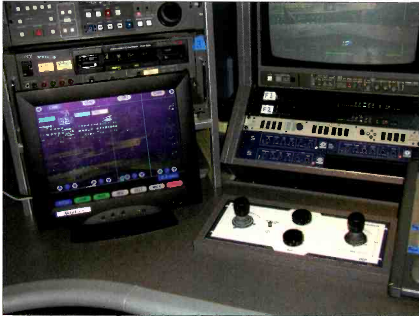
A Vinten AutoCam camera control system with a flat-panel touchscreen display in AMEX's broadcast department.
