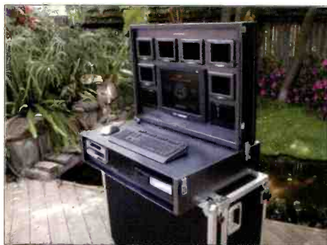
The Journeyman, a virtual studio in a box, has a 17" flat-panel LCD control monitor; eight individually assignable, 5.6" LCD monitors; and a control PC, keyboard and mouse.
