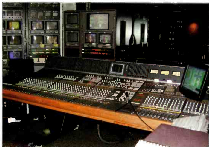
The ability of the Calrec Alpha 100 console to handle 5.1 surround sound will become increasingly important as NBC expands Studio 3A's use to entertainment and sports.
