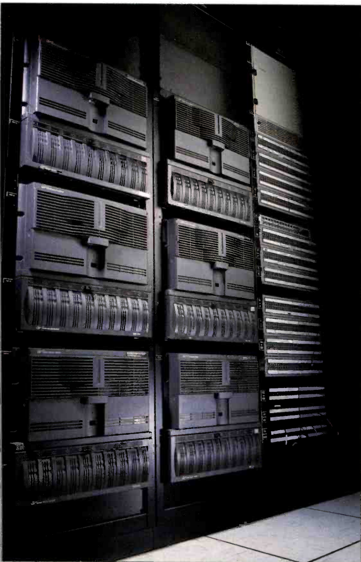
ASCN uses six Grass Valley Group Profile XP Media Platform systems for playout, interfaced with the network's automation system, tape machines and other systems for easy expansion.
