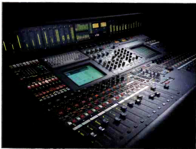
This Neve Libra Live II exhibits a combination of bar graph, ballistic VU and flat-panel displays.
