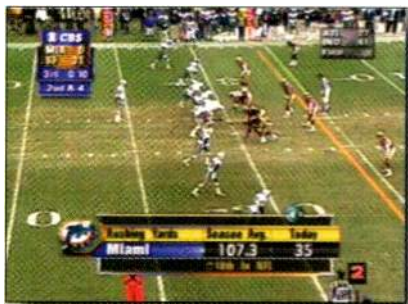
Fox box in upper left corner provided by SGI O2, lower banner provided by Chyron Infiniti!, and Sportvision's first-and-ten line provided by SGI equipment. The score in the upper right is a linear key, usually provided by a Digital PC Codi.
