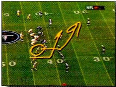
Color announcer draws on stylus touch pad overlaid on a monitor. This used to be performed with a light pen. The key is generally performed with a Chyron Codi.
