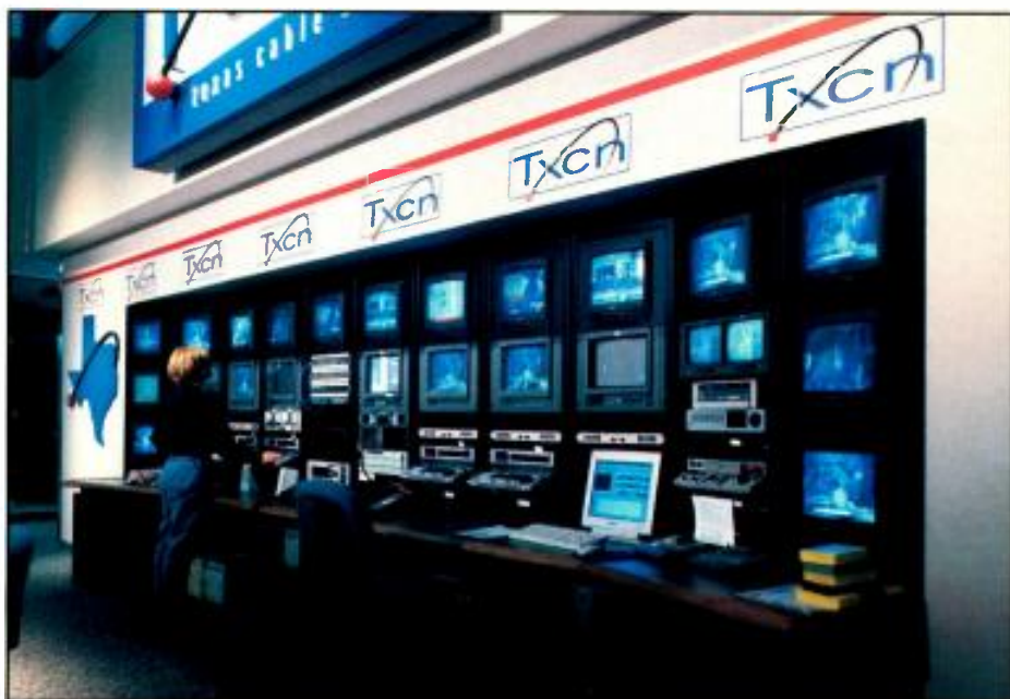
MPEG splicing helps stations maintain picture quality by avoiding decompression-recompression cycles in editing systems like the one at Texas Cable News (shown above). Photo courtesy Concept: Benson & Rice.
