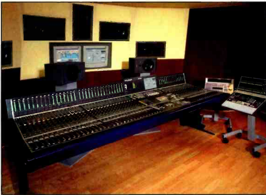
Virtual Surround Panning (VSP) technology in Studer's D950S, shown above, is utilized in mix-downs to create a realistic-sounding envelopment by integrating monophonic sources.
