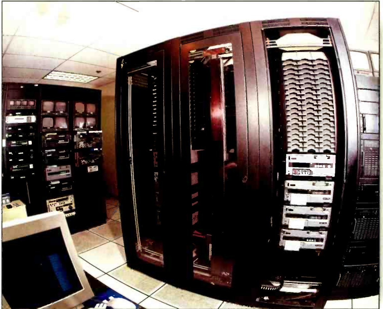
Ackerly's CentralCasting employs a TiltRac V-300 Video Library Manager for its long form and archived program for its regional stations.
