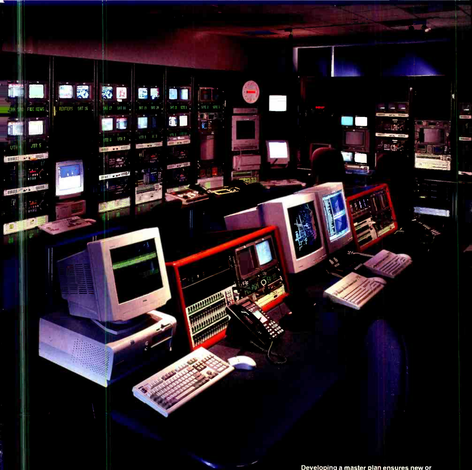
Developing a master plan ensures new or renovated facilities meet current and future demands. A satellite feedroom is shown here. Photos by Aker/Zvonkovic Photography, Houston.
