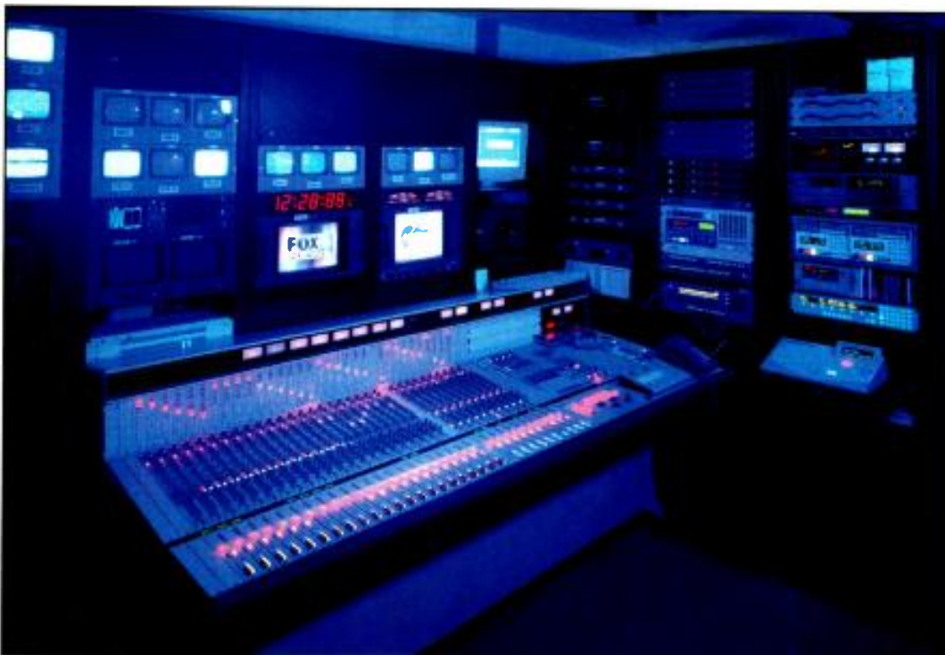
The audio control room features a Wheatstone TV-80 analog audio console with over 350 inputs available to 22 mono channels and 10 stereo channels.
