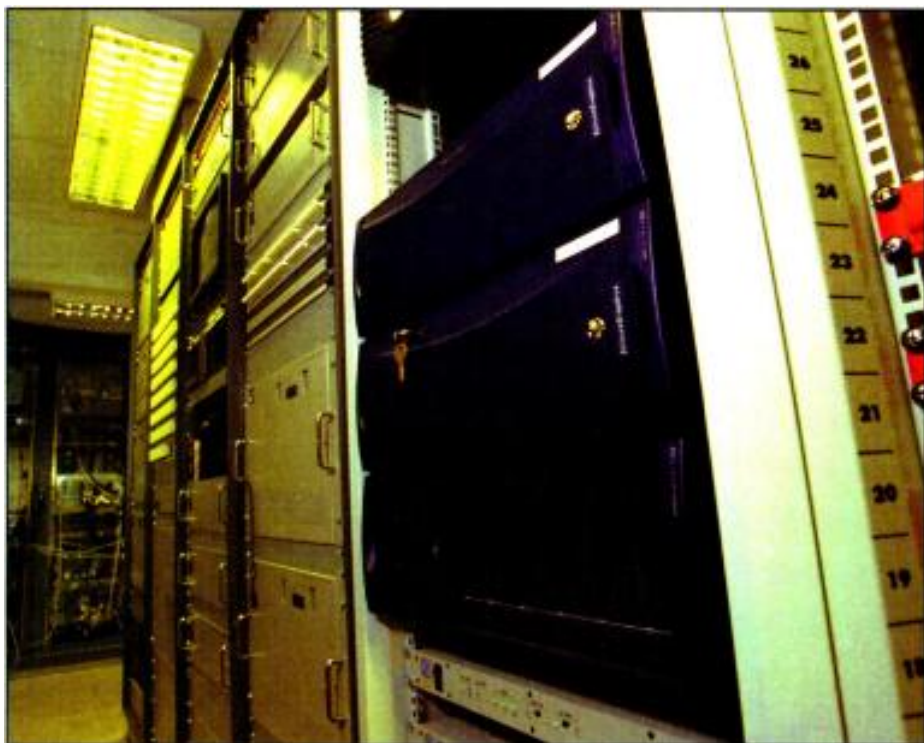
SVT uses SGI Media Servers like the one shown above to transfer news stories as DVCPRO25 .dif files between their headquarters in Stockholm and regional facilities. The systems are linked with an E-3 34Mb/s microwave WAN.
