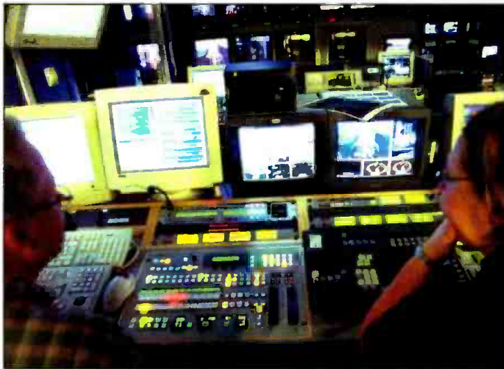
SVT's Hawry's automation software, shown above, provides for selection and playback of clips, starts the countdown clock and controls CG, switching and still store equipment.
