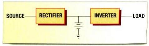
Figure 2. In an online configuration, incoming power is fed to the system's battery at all times, providing an effective low pass filter.
