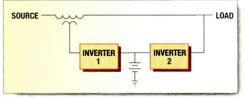
Figure 4. In a delta conversion configuration, a second two-way inverter can either add voltage to the tranformer tap or act as an additional load to lower the current out.
