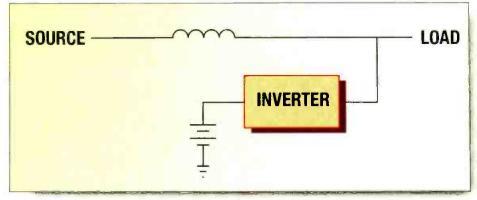
Figure 3. In a single conversion UPS, separate rectifiers and inverters are replaced by an inverter/rectifier that passes power both to the battery and back out again to load.
