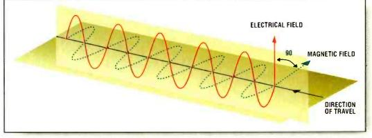
Figure 2. Electromagnetic waves travel as an electrical wave and a magnetic wave on two seperate planes at a 90 degree angle.
