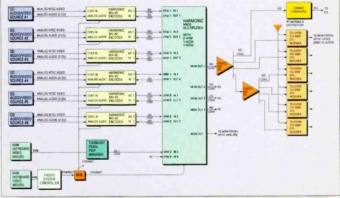
Paxson's WCPX-DT is multicasting six channels of progamming in its allotted 6MHz. The stations employs Harmonic encoding and multiplexing equipment, Evertz DAs and Thomcast's Pearl PSIP manager.
