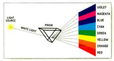
Figure 1. When passed through a prism, white light can be split into spectral colors.
