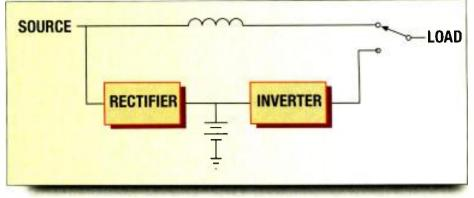
Figure 1. Lower-end UPS systems are likely to employ an offline UPS configuration, which simply opens the path from the battery in the event of a power failure.
