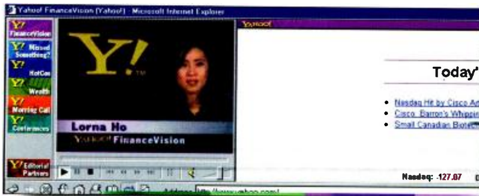
Yahoo's FinanceVision webcasts are compressed by a Windows Media Encoder for either 300K/100K or 56K modem speeds. The service offers stock market and other financial news updates every half-hour.
