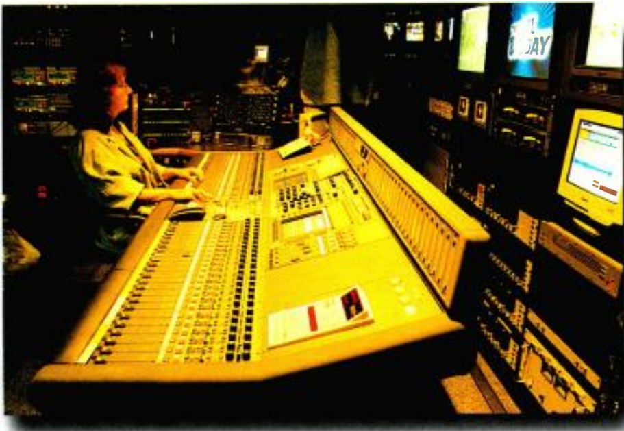
CBS Audio Engineer Mary Cody at the AMS Neve Libra Live broadcast production console within CBS's control room #43 in its New York headquarters. Broadcasters should carefully consider their audio needs before purchasing an analog or digital console. Photo courtesy of AMS Neve.
