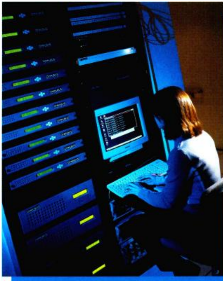
A facility-wide Omnibus automation and control system provides on-air media management, as well as supporting the dubbing and playout of spots and interstitial. A Grass Valley M2100 can handle both SD and HD playout channels under Omnibus control.
