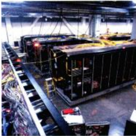
Ongoing integration work on several RIBs at Sony's integration facility in San Jose.
