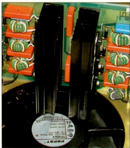
Fan blades and cooling fins must be kept clean and clear of dust and dirt. (Courtesy of Continental.)
