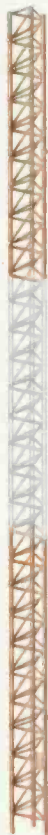
Figure 1. Additional bays focus more of the radiated signal to the horizon and add gain to the system.
