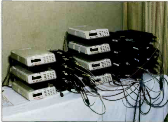
During Super Bowl week last January, MJI Broadcasting established an ad-hoc network of stations for sports-talk programs fed directly from Phoenix via this ISDN codec/TA setup. (Photo courtesy of Comrex Corporation.)
