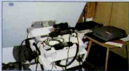
Portable uplink feeding the Inmarsat AOR-E satellite through a window in a Tuzla, BiH apartment providing POTS or ISDN connectivity to the U.S. Codec and fax machine are on tables at rear.
