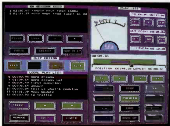
The audio upload/editor screen from NewsRoom , an integrated, PC-based digital news system from Computer Concepts. A "virtual VU meter" helps users make the transition from traditional systems.
