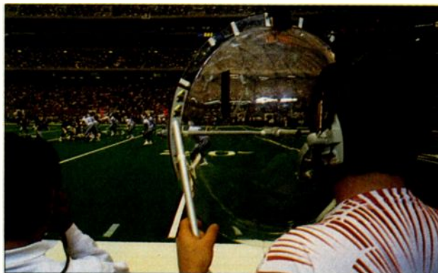
One of the parabolic microphones used on the field to create the stereo sound of Dallas Cowboys radio broadcasts. Both the microphone and its operator's headset feeds to/from the control booth are wireless, allowing easy movement along sideline.
