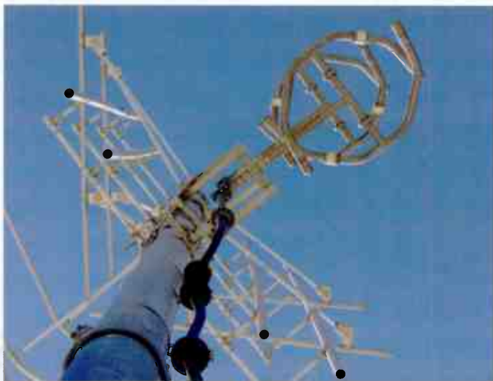
The KCSN (highly directional) booster antenna.
