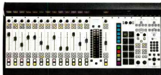
The Axia Fusion is a modular console available in frame sizes that support 8 to 40 faders in single or multiple linked frames.
