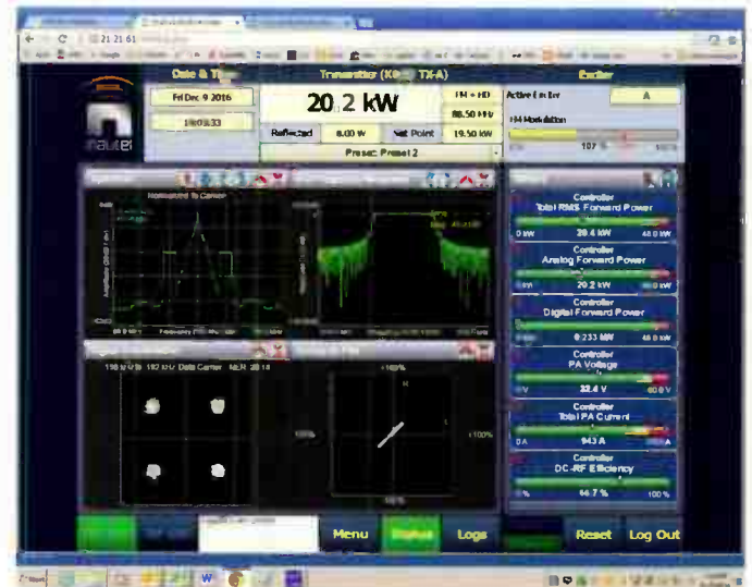
The Nautel AUJ home page shows the basics such as the modulation level, the power level, the preset in use and user-selectable metering parameters. In this view we also see the RF spectrum, the MER constellation and a Lissajous pattern indicating left vs right audio.
