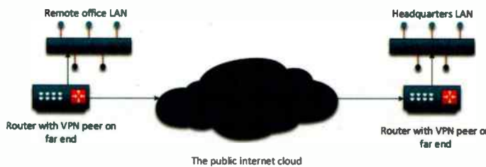
Fig. 3: Main office and remote office connected via the public internet but using VPN peers.
