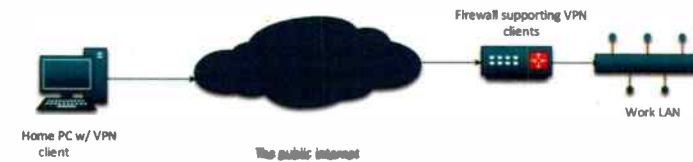
Fig. 1: Typical remote user with VPN client on local machine.
