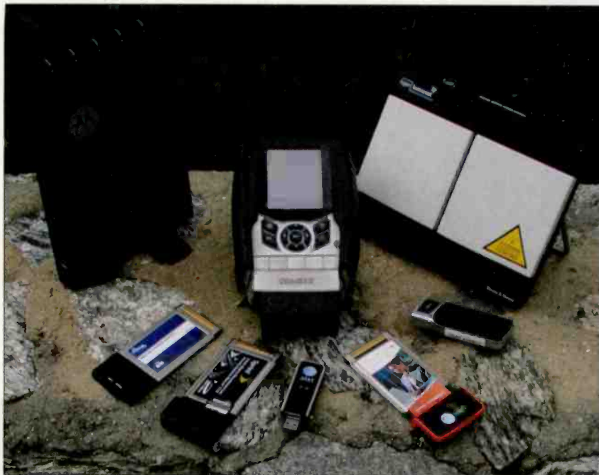
Comrex Access (center) with Wimax modem (left) Inmarsat terminal (right) and a variety of 3G and Wi-fi modems (front)
