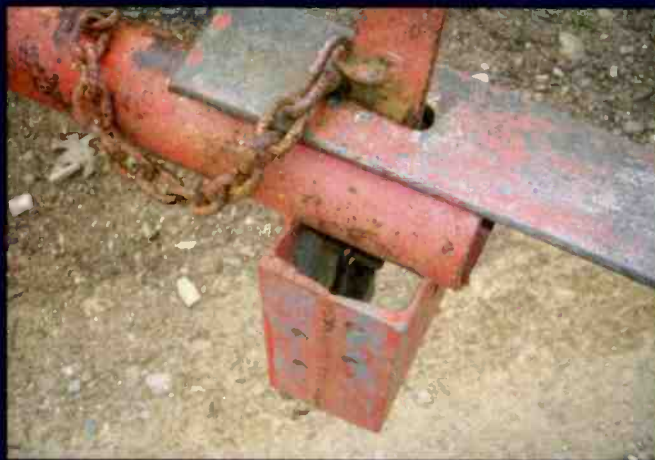
A cover around a padlock makes it harder for a thief to cut it.
