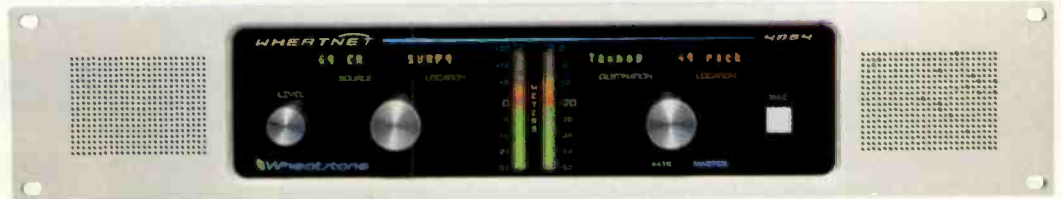
The Wheatnet Switch is an X-Y router controller for the Bridge.
