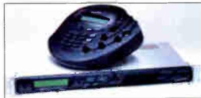
As a 15kHz POTS codec, the Matrix can connect with all Comrex POTS codecs, and with the optional ISDN module, the Matrix is compatible with most ISDN standards. When the remote site has no phone line, the optional GSM module allows the Matrix to transmit 7kHz audio with an internal GSM wireless phone. Along with the full line of Comrex codecs and telephone hybrids, the Matrix will help your station broadcast great-sounding audio from anywhere.
