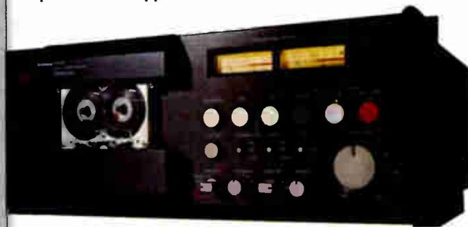
The TCD 910 was intended to replace reel-to-reel and cartridge machines in many applications. Touting its high specs, the deck was "capable of producing tapes at sound and silence levels beyond that required by broadcast and studio requirements." It offered a real-time counter and auto-locator functions.
