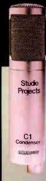
The Studio Projects C1 is a cardioid condenser microphone with a 1.06" capsule, low-noise FET amplifier and balanced, transformerless output circuitry. It features a switchable 10dB pad and a 6dB at 150Hz high-pass filter. It includes a shock-mounted elastic suspension, foam wind screen and a hard-side carrying case. The mic's frequency response is from 20Hz to 20kHz with a maximum input of 142dB. The output impedance is less than 200Ω. It operates on phantom power.
