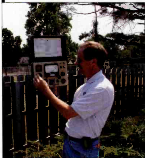
Use a field strength meter to not only take monitor point readings, but also to track problems due to reradiation.
