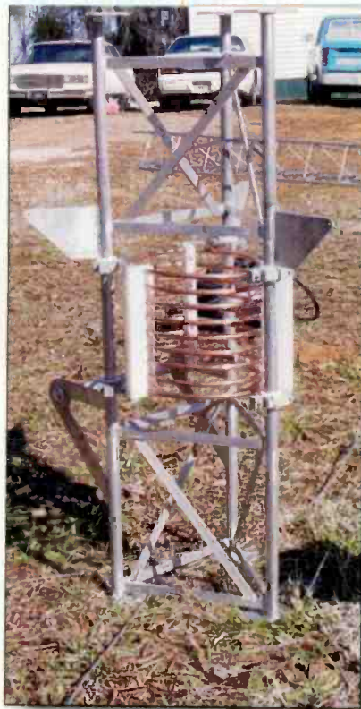
Detail of the EH antenna phase-shift network.
