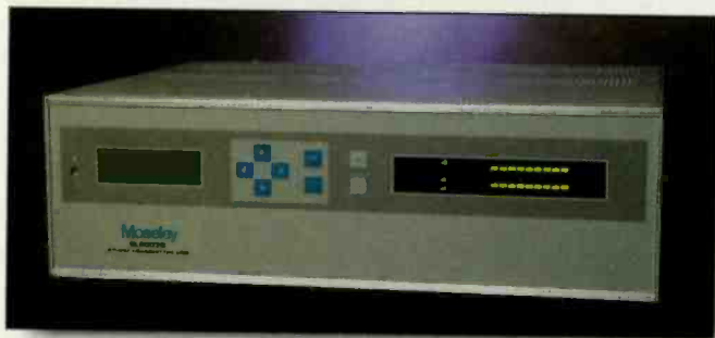
Quadrature amplitude modulation has made it possible to send four linear digital audio channels over conventional STL paths and frequency spacings.
