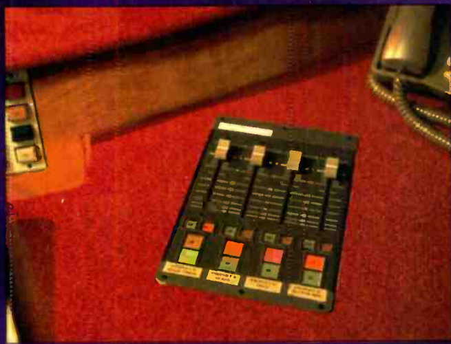
The Vadis D.C. four-fader mixer delivers considerable control in a minimal space.
