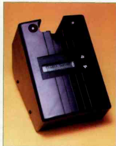
The base station recharges the PPM and downloads its data.
