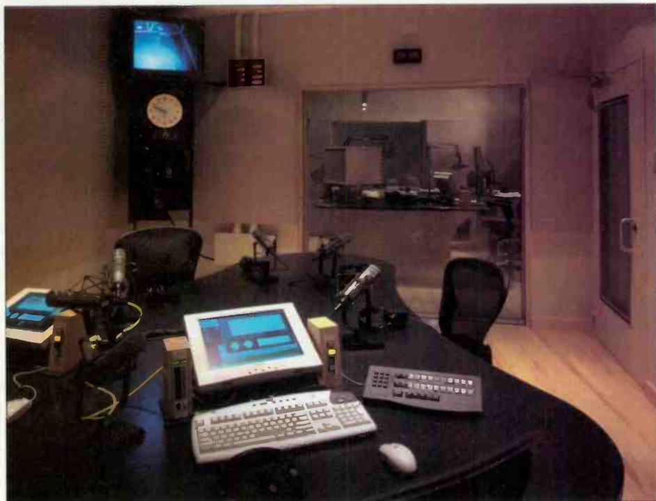
The talk studio should be comfortable for guests and still provide the host all the needed tools. Above, the computer monitor is used for call screening.
