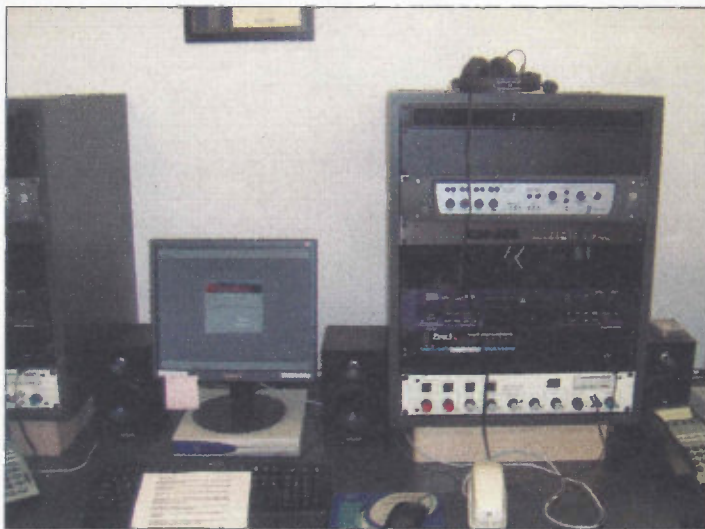
The newsroom is a collaborative workspace encircled by audio editing and news production workstations like this one. Each position has a Protocols 002 system as well as the Newsboss workstation.
