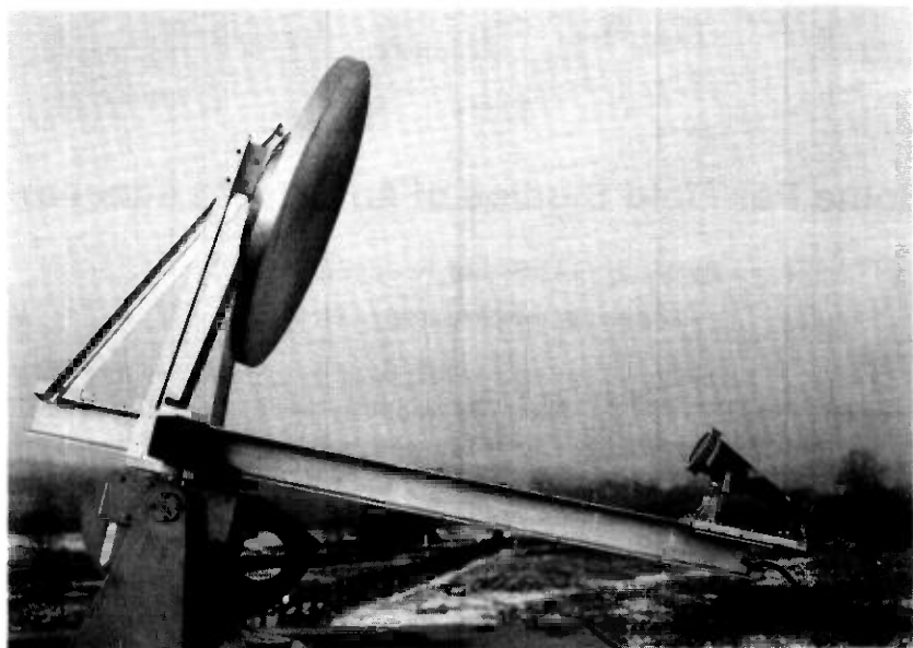
Fig. 1—Offset launcher. The 76-cm (30-in.) diameter reflector is a numerically machined section of a paraboloid. Reflector focal length is 115.7 cm and it is fed, in this instance, by a 28.5-GHz dual-mode horn with a polarizer.
