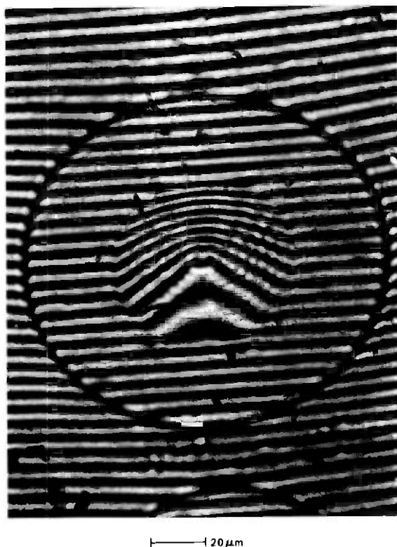
Fig. 7—Microinterferogram of linear refractive-index profile fiber showing index depression in center.
