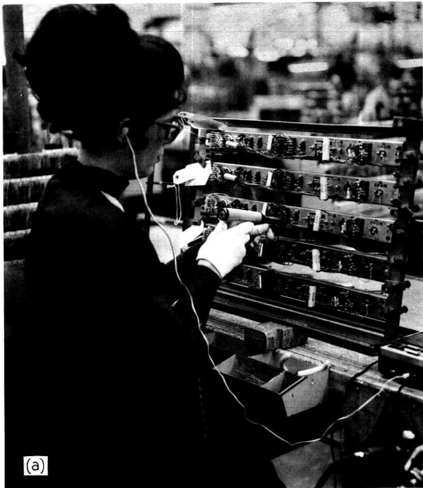
Fig. 3a—Wireman on production line at Western Electric Company plant in Oklahoma City. The wireman is fabricating crossbar-4 equipment from the computer-spoken wire list.
