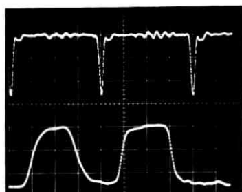
Fig. 18—(a) Information gate. (b) Information gate switching: top trace, output; bottom trace, information input (2 ns/cm, 2 V/cm).
