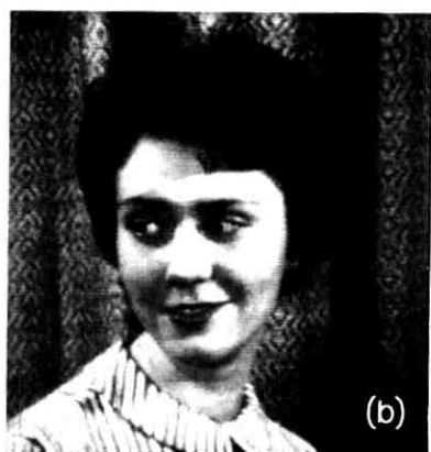
Fig. 5—(a) 10 bits per picture-element; (b) Reconstruction of (a) by means of the Hadamard basis, using 2 bits per picture-element; (c) Reconstruction of (a) by means of differential PCM, using 3 bits per picture-element.
