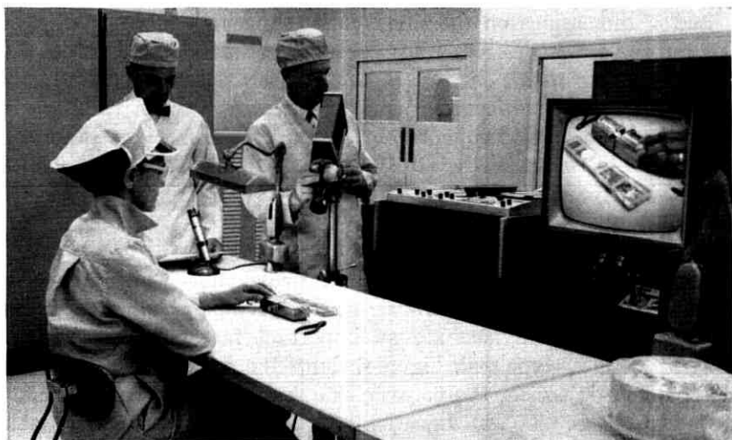
Fig. 4—Stacking of a mica capacitor being videotaped and viewed simultaneously on TV screen.
