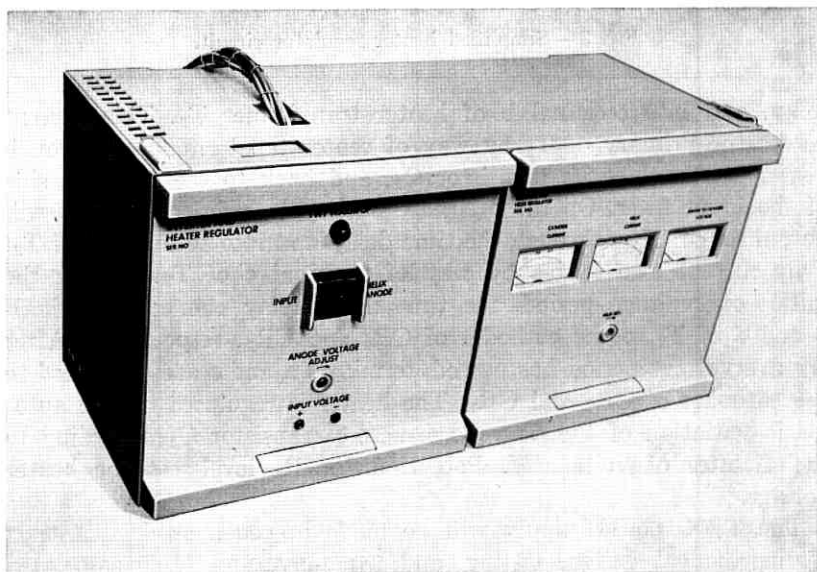
Fig. 4 — TWT power supply.
