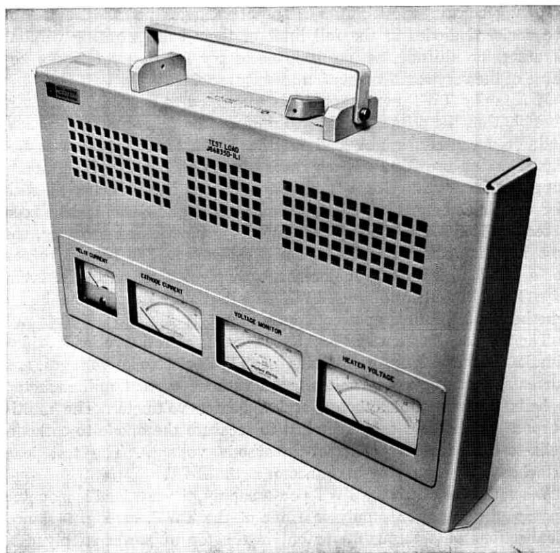
Fig. 8 — Test load for the TWT power supply.
