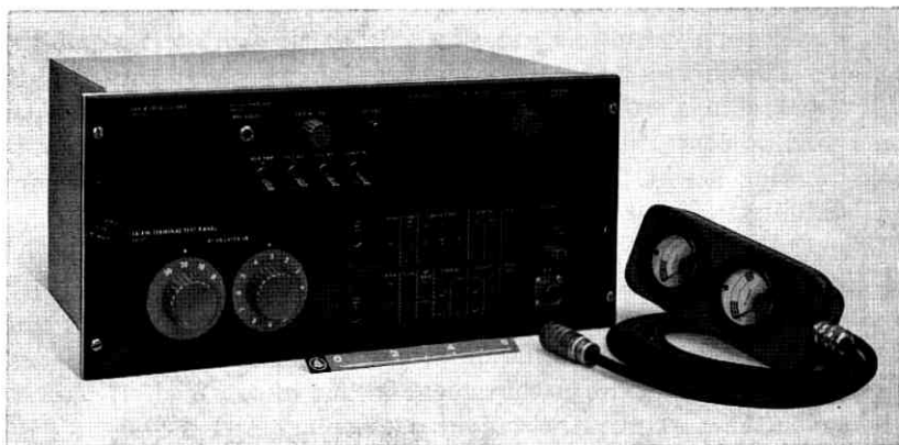
Fig. 10 — 3A FM terminal test panel.
