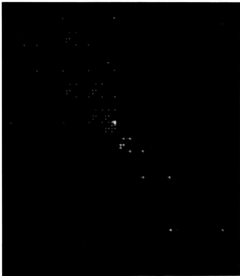
Fig. 11 — Focal plane intensity distribution with modulators set at E = 10 dB.
