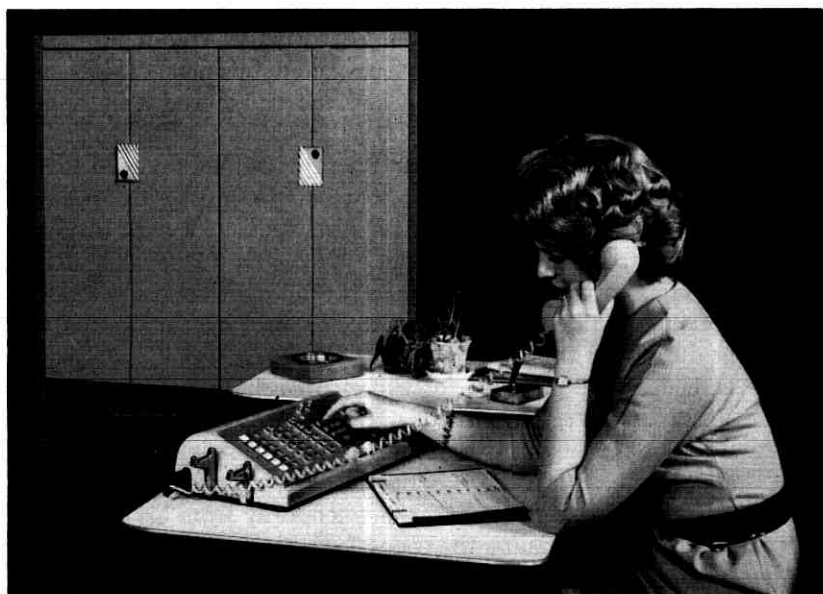
Fig. 47 — No. 101 ESS 200-line switch unit and attendant's console.
