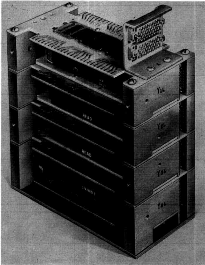
Fig. 34 — The No. 1 ESS ferrite sheet module has a capability of 2048 words of 24 bits each or a total of 49,152 bits. Four such modules are used in each call store.
