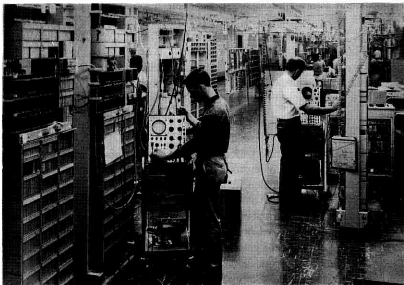
Fig. 39 — Western Electric Company manufacturing operations: monorail area — frame testing.
