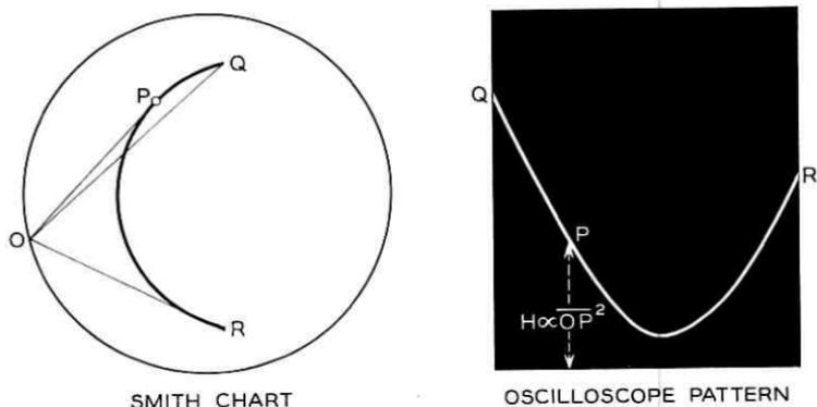
Fig. 7 — Relation between impedance locus and oscilloscope pattern.
