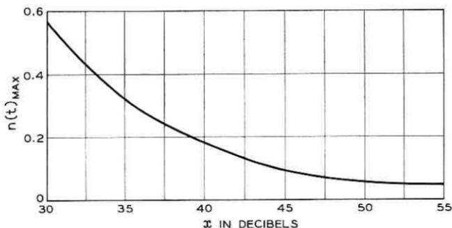
Fig. 26 — Peak crosstalk interference as a function of 1.544-mc crosstalk loss.
