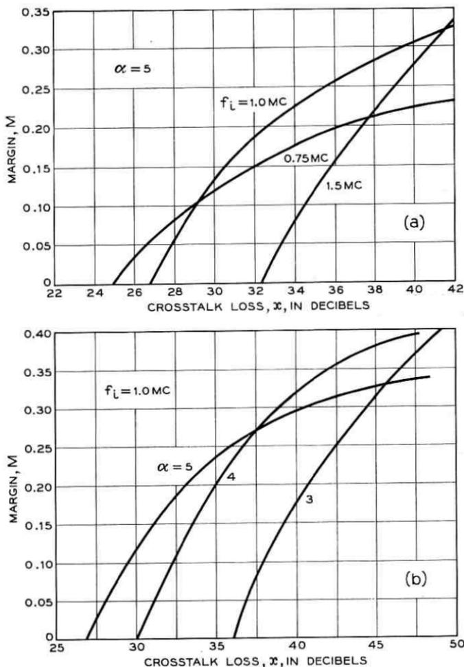
Fig. 7 — Margin as a function of  $x$  for (a) various  $f_i$  and (b) various  $\alpha$ .
