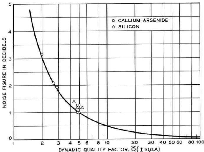
Fig. 12 — Measured noise figure versus measured dynamic quality factor  $\tilde{Q}$  ( $\pm 10\mu a$ ).
