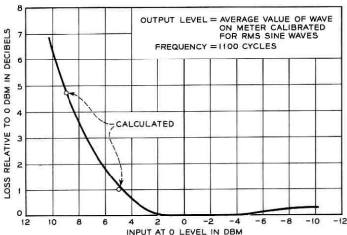
Fig. 17 — Measured signal compression vs input signal level.
