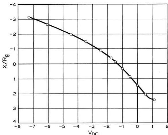
Fig. 13 — Small-signal reactance versus bias voltage (Locus III).
