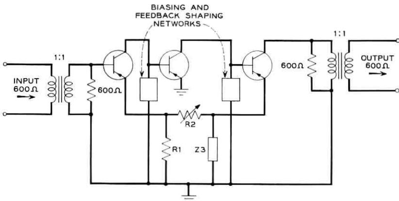
Fig. 3 — Simplified circuit of emitter feedback amplifier.
