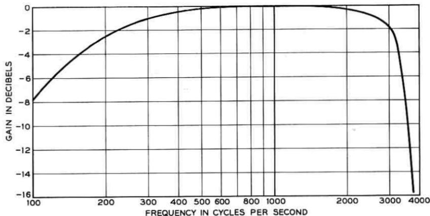
Fig. 6 — Typical bandpass characteristic of the channels.
