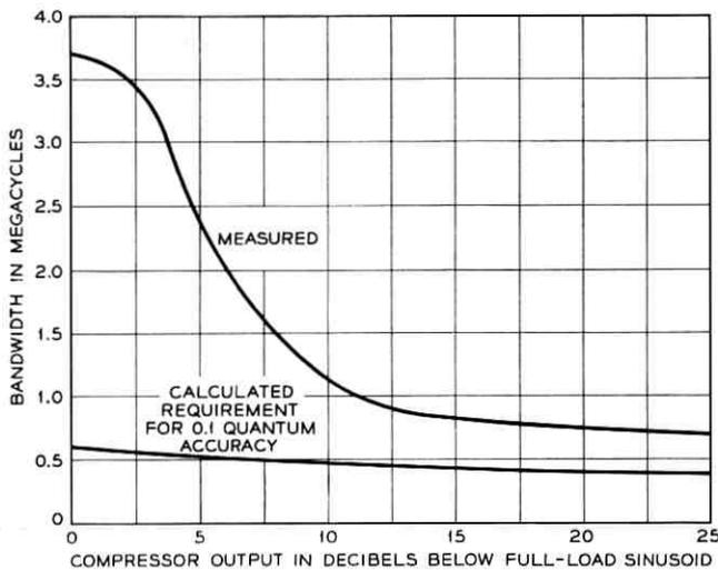
Fig. 18 — Compressor output signal vs compressor bandwidth.
