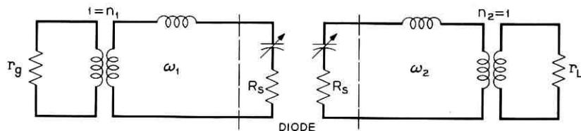
Fig. 2 — Equivalent circuit of the parametric amplifier.
