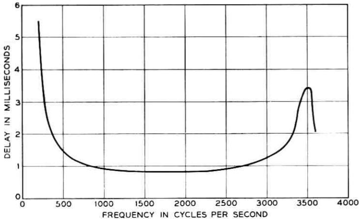
Fig. 20 — Typical channel delay-frequency characteristics of A5 bank.
