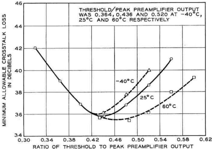
Fig. 61 — Typical crosstalk vs threshold.
