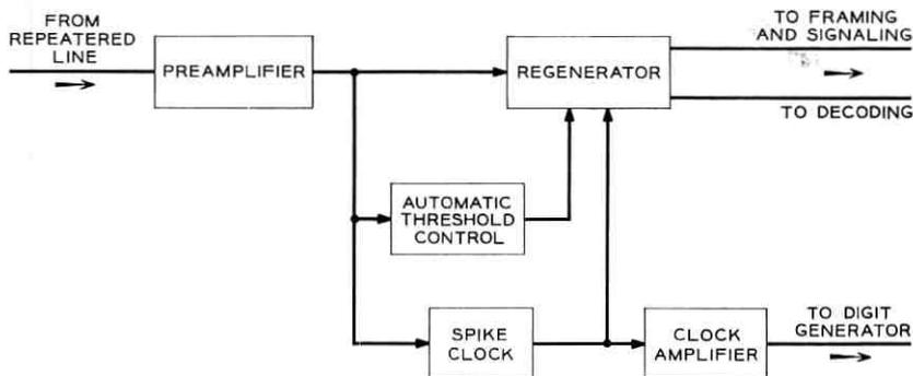
Fig. 52 — Block diagram of receiving repeater.
