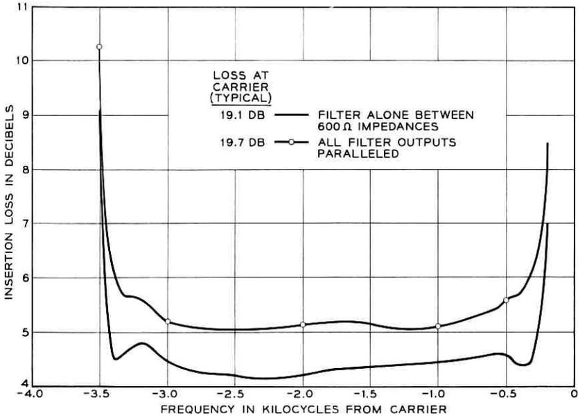
Fig. 17 — Typical pass-band characteristic of a channel filter.
