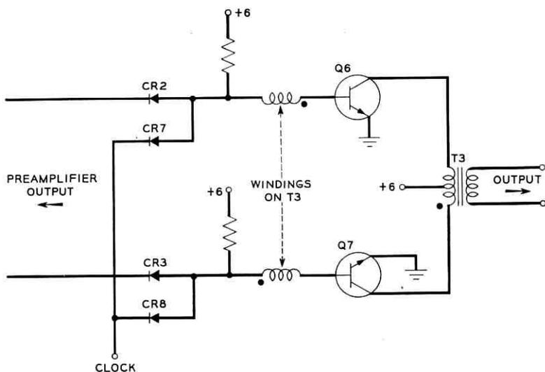
Fig. 34 — Regenerator circuit.
