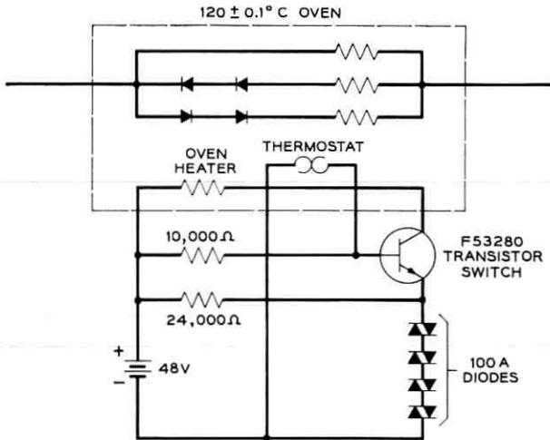
Fig. 17 — Increased thermostat life via transistor gain.
