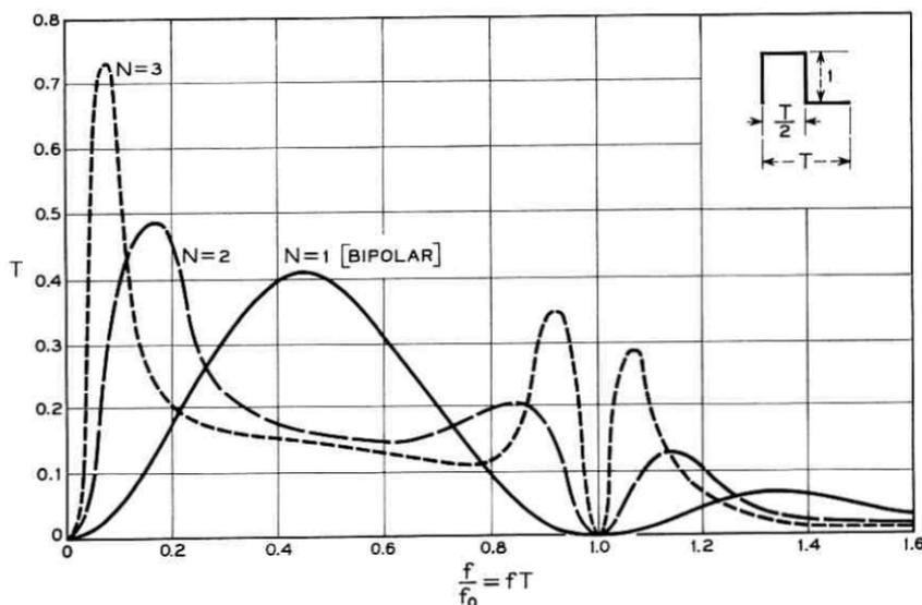
Fig. 12 —  $N$  pulse power spectra.
