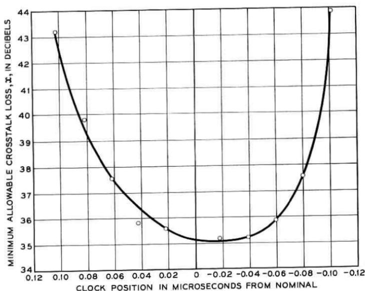
Fig. 55 — Typical measured effect of clock phase on crosstalk performance.
