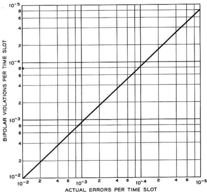
Fig. 43 — Comparison of error rates, actual and as indicated by error meter, for errors generated by exposing working repeater to random noise.
