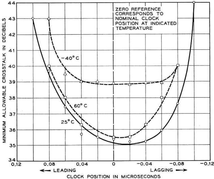
Fig. 60 — Typical crosstalk vs clock position.
