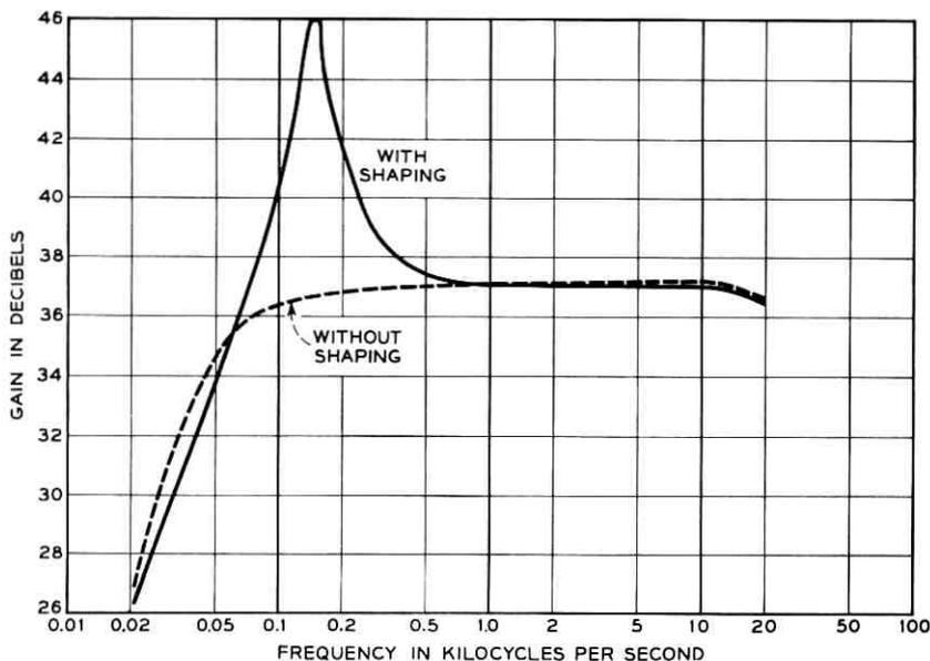
Fig. 8 — Closed loop voltage gain of the amplifier.
