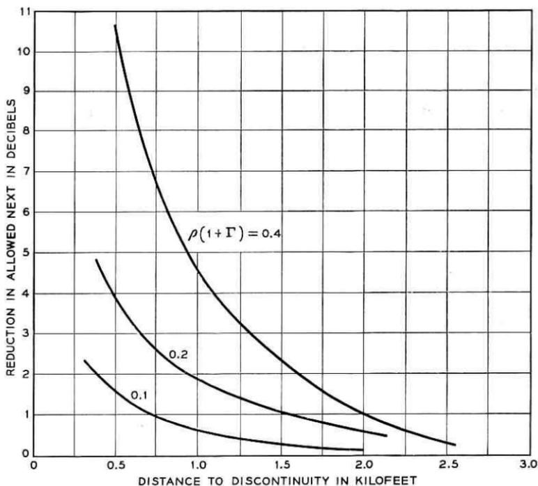
Fig. 35 — Effect of reflected signals on NEXT performance.
