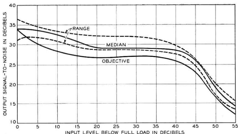
Fig. 4 — Plot of signal-to-noise measurements over 24 channels.
