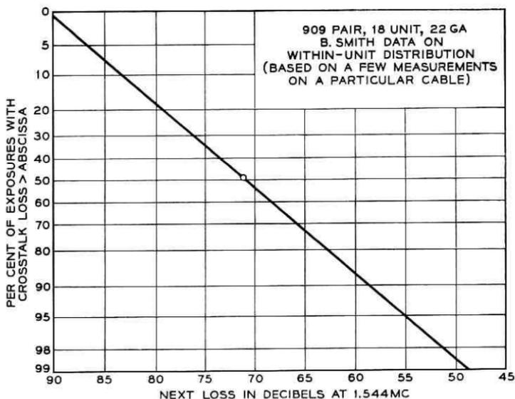
Fig. 2 — Distribution of near-end crosstalk loss.
