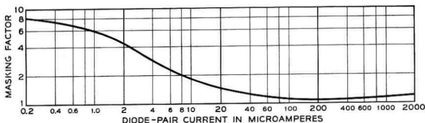
Fig. 15 — Factor by which per cent diode-pair voltage variations are reduced by resistance masking.
