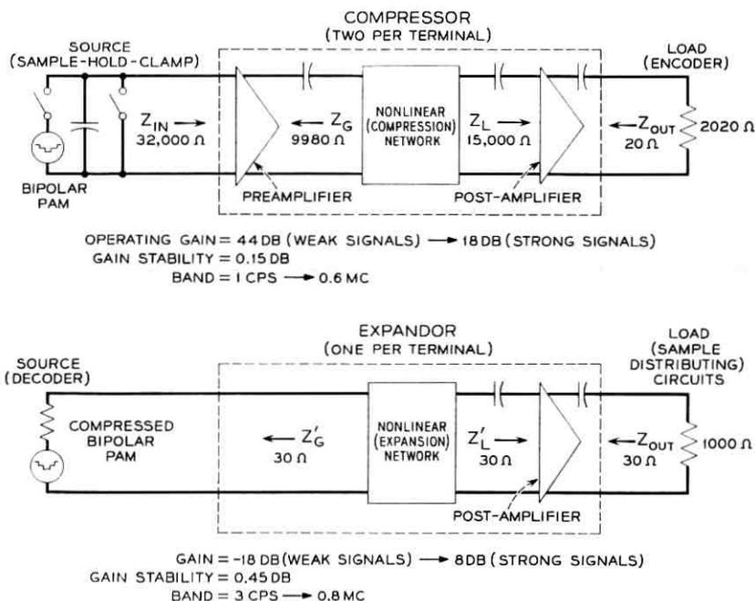
Fig. 7 — Block diagrams showing compressor and expander.
