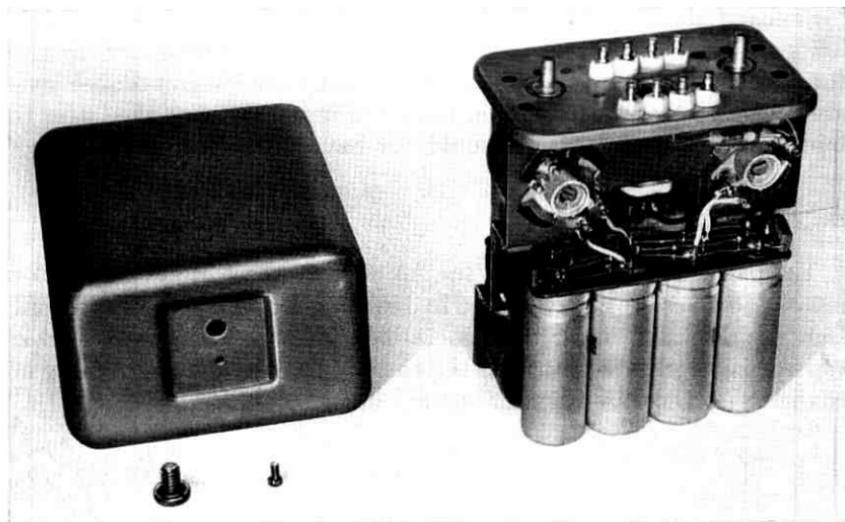
Fig. 15 — Crystal channel filter assembly comprising a transmitting and a receiving unit.
