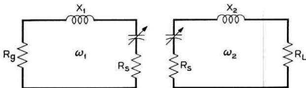
Fig. 3 — Elimination of the transformer in the equivalent circuit of Fig. 2.
