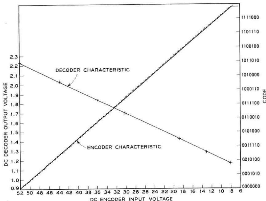
Fig. 28 — The encoding and decoding dc transfer characteristics.
