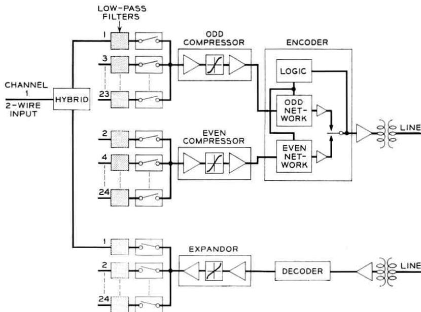
Fig. 1 — Experimental PCM system — speech portion of terminal.
