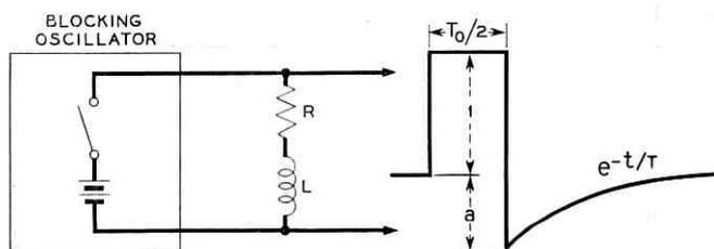
Fig. 19 — Simplified blocking oscillator operating into inductive load.
