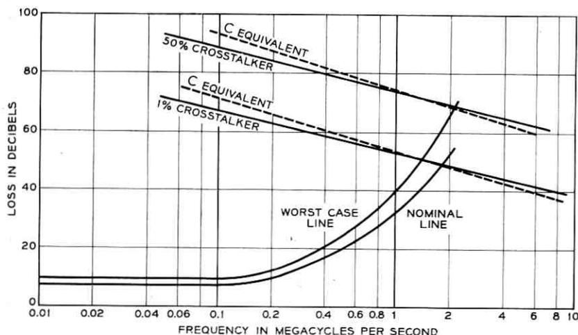
Fig. 9 — Line loss and crosstalk loss.
