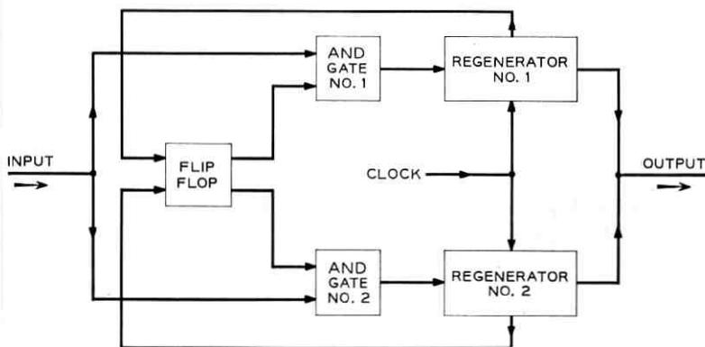
Fig. 51 — Block diagram of transmitting repeater.
