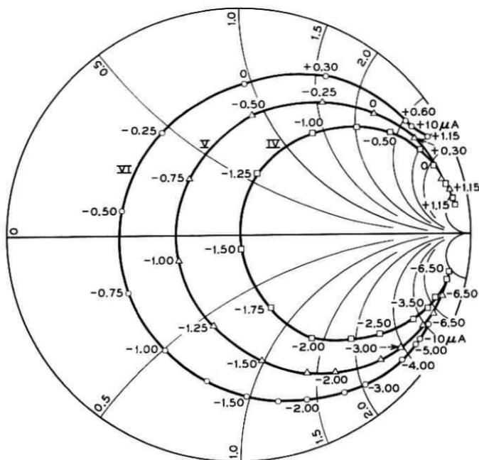
Fig. 10 — Impedance loci of a silicon mesa diode.
