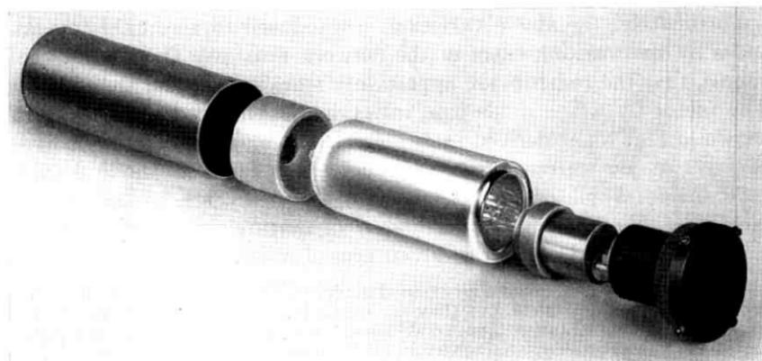
Fig. 16 — Temperature-controlled oven.
