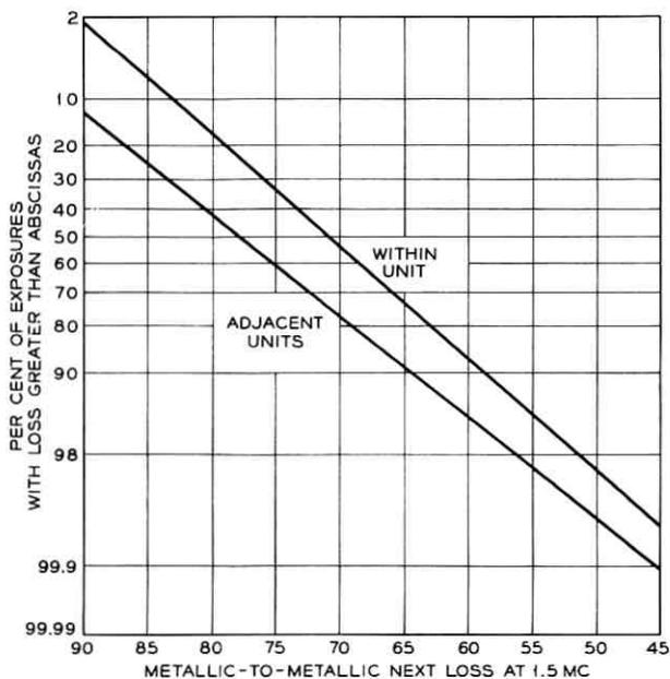
Fig. 7 — Preliminary near-end crosstalk loss distribution.
