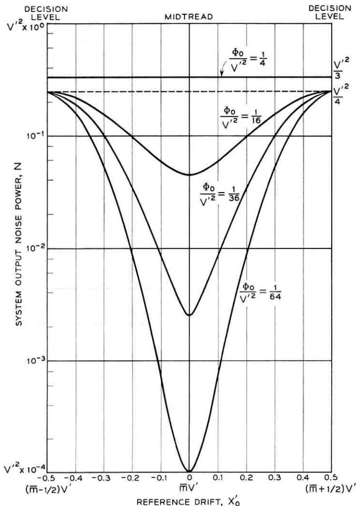
Fig. 9 — System output noise power vs reference drift  $X_0$ . The input noise power as a fraction of the step size  $V'$  is taken as a parameter. The reference drift is shown to vary between any two adjacent decision levels.
