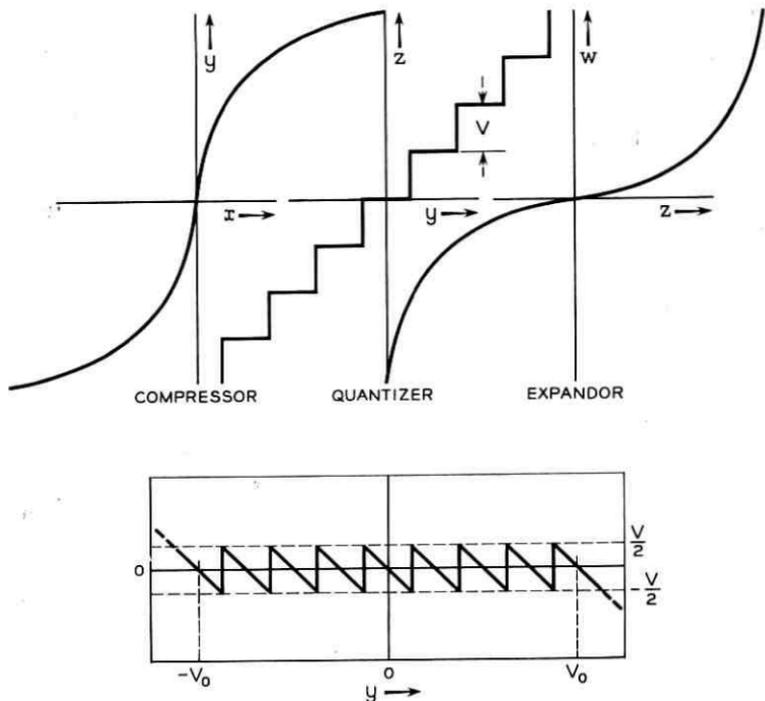
Fig. 7 — Transmission characteristics of the compressor, quantizer, and expander. The quantizer transmission is decomposed into the sum of a linear term plus a periodic sawtooth function.
