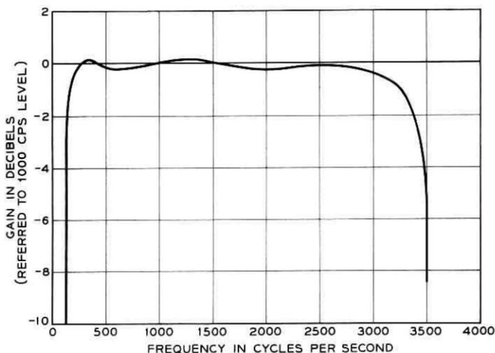
Fig. 19 — Typical channel gain-frequency characteristic of A5 bank.
