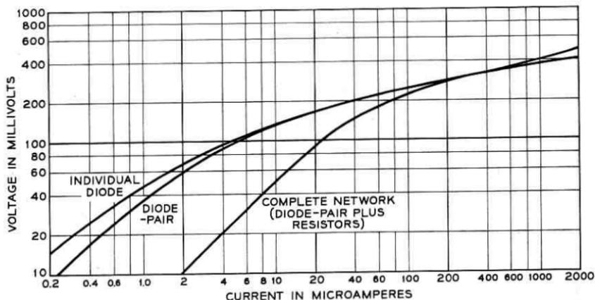
Fig. 11 — Comparator voltage vs current characteristics (diodes at 120°C, resistors at 25°C).
