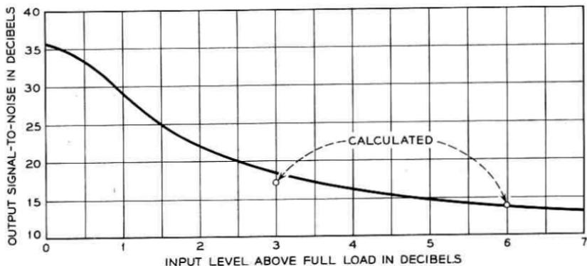
Fig. 18 — Measured signal-to-noise ratio vs input signal level for signals above full load.
