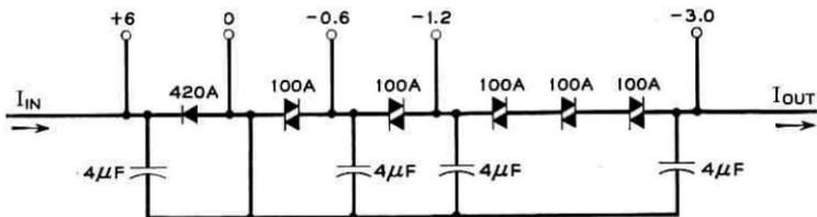
Fig. 39 - Twin repeater power unit.
