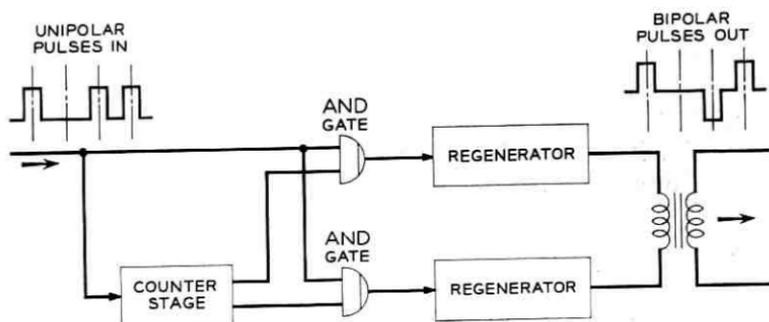
Fig. 11 — Bipolar converter.
