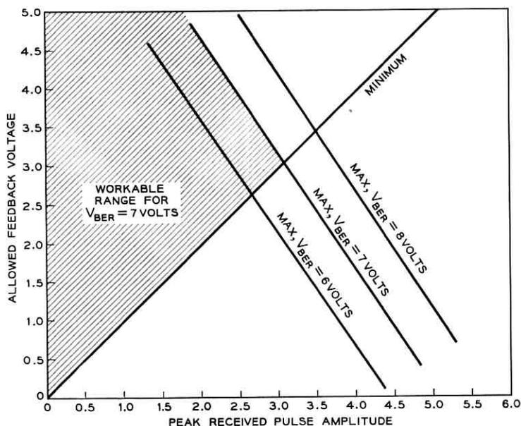
Fig. 37 — Maximum and minimum allowed feedback voltage.
