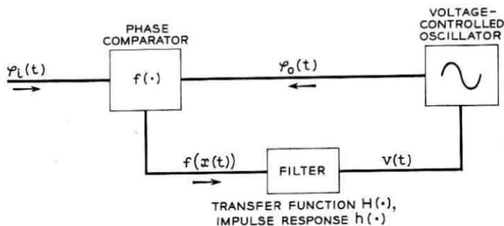
Fig. 1 — Phase-controlled loop.
