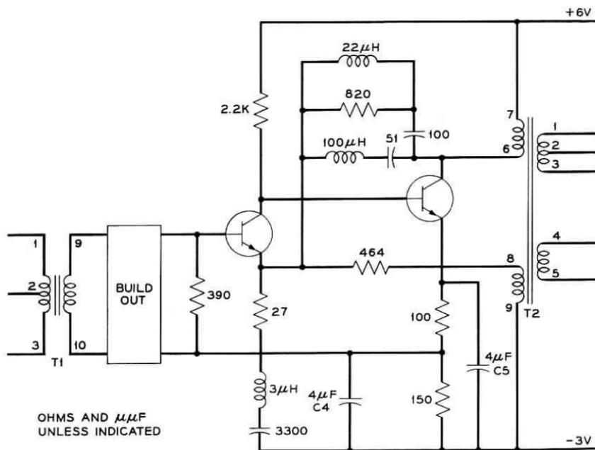
Fig. 14 — Repeater preamplifier circuit.
