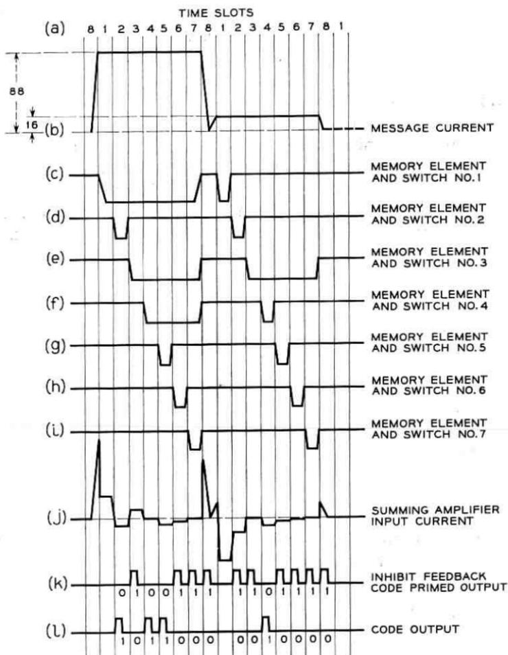
Fig. 20 — The encoding process.
