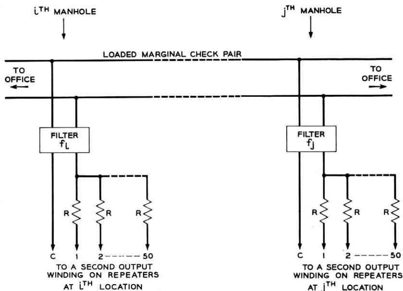
Fig. 44 — General plan for marginal checking 25 two-way systems.
