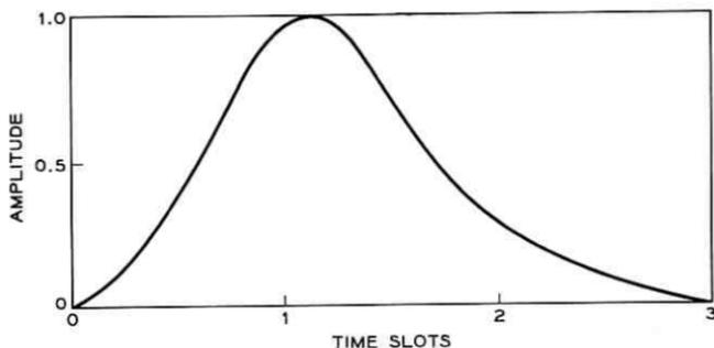
Fig. 9 — Pulse shape resulting from transmission through  $G(jf)$ .
