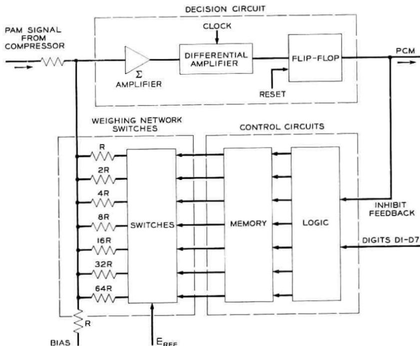
Fig. 19 — Sequential comparison encoder.
