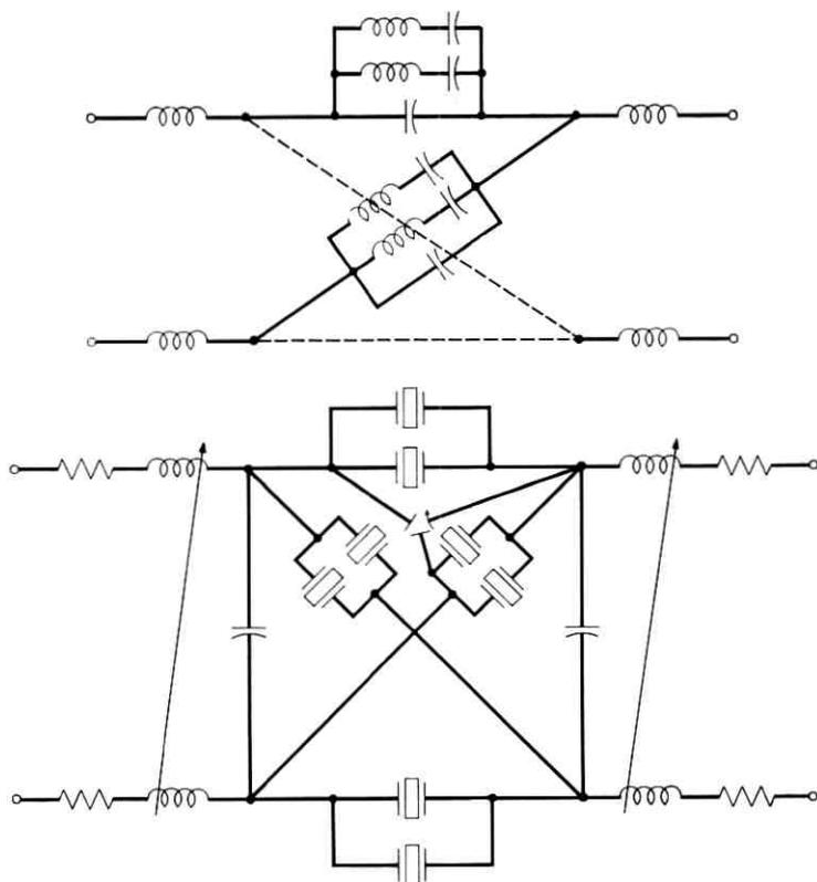
Fig. 14 — Configuration of a crystal channel filter.
