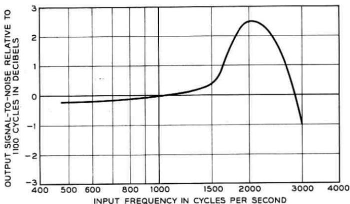
Fig. 5 — Plot of signal-to-noise ratio vs input frequency.
