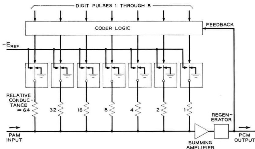
Fig. 4 — Simplified block diagram of network coder.
