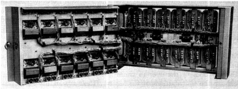
Fig. 13 — A5 bank with hinged door open showing rear of modem units and the filters mounted on rear frame.
