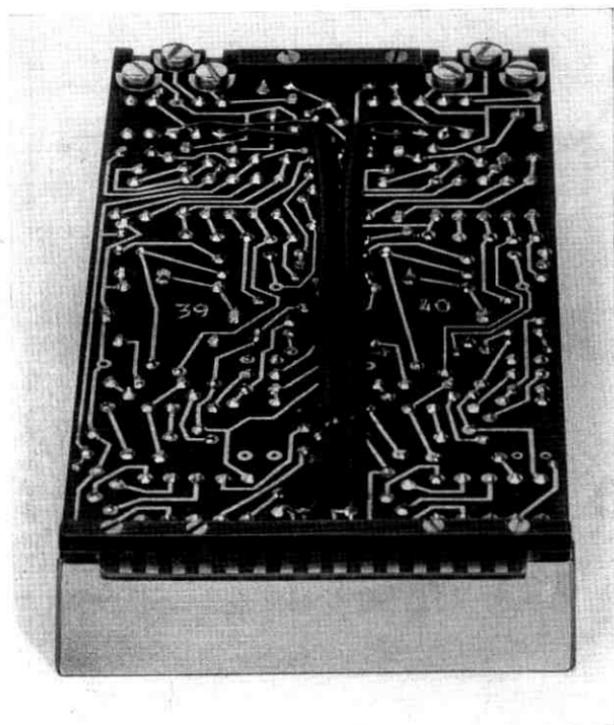
Fig. 50 — Printed wiring of repeater.
