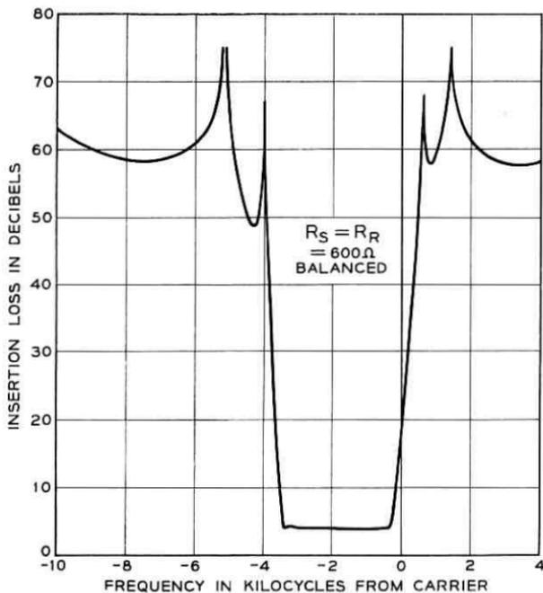
Fig. 16 — Typical loss-frequency characteristic of a channel filter.
