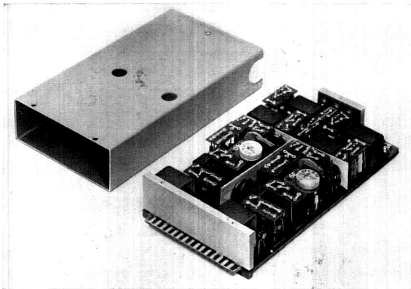
Fig. 48 — Experimental PCM repeater, cover removed.
