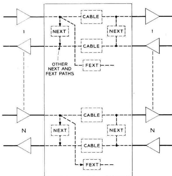
Fig. 6 — "Channel" for  $N$  PCM systems.
