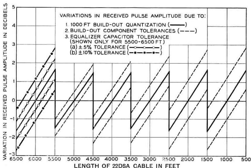
Fig. 21 — Variations in amplitude vs cable length.
