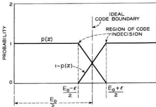
Fig. 27 — Model for the study of the effect of transition uncertainty on quantizing noise.
