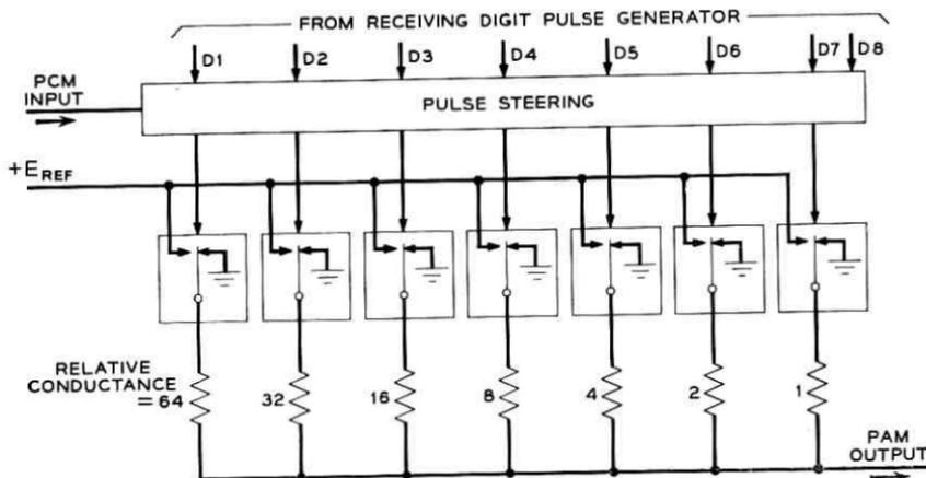
Fig. 5 — Simplified block diagram of decoder.
