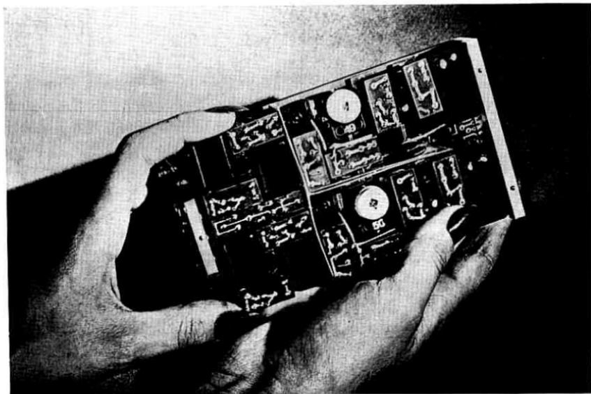
Fig. 12 — Experimental two-way repeater with cover removed.
