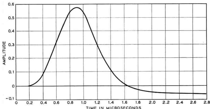
Fig. 20 — Pre-amplifier output including effect of RL network.
