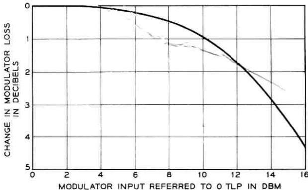
Fig. 21 — Typical channel overload characteristic showing modulator limiting.
