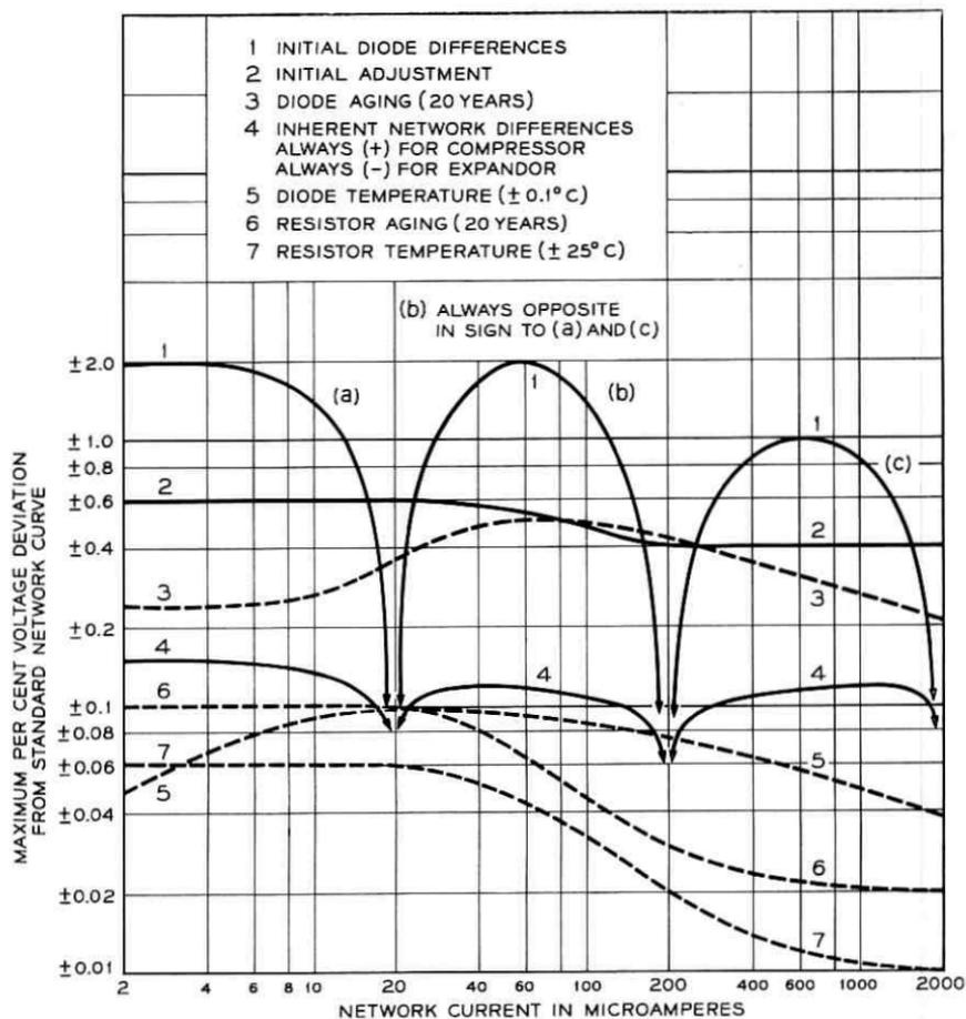
Fig. 12 — Comandor network tolerances that contribute to mistracking.
