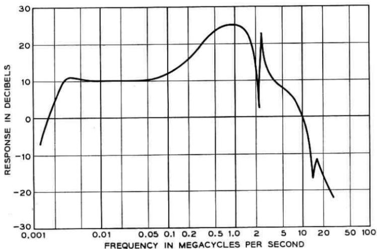
Fig. 15 — Measured preamplifier response.
