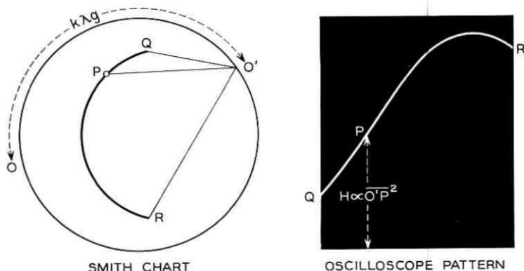
Fig. 8 — Shift of probe position and oscilloscope pattern.
