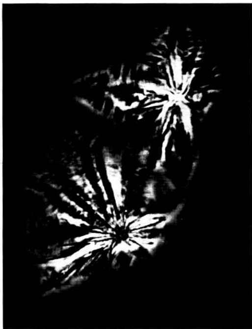
Fig. 2 — Multilayer dendrites in the same preparation as in Fig. 1. (Phase-contrast microscopy; magnification of original photograph 600X.)
