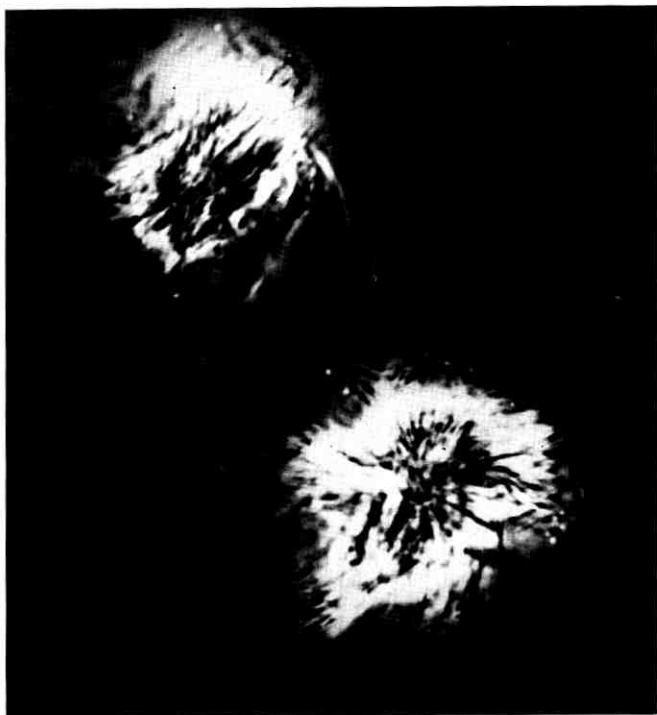
Fig. 3 — Typical compact crystal formations of polyethylene formed at 85°C from 1 per cent xylene solution; the crystals are in their mother liquor. (Phase-contrast microscopy; magnification of original photograph 1000 \times .)
