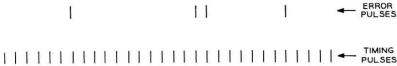
Fig. 2 — Method of error recording on magnetic tape.
