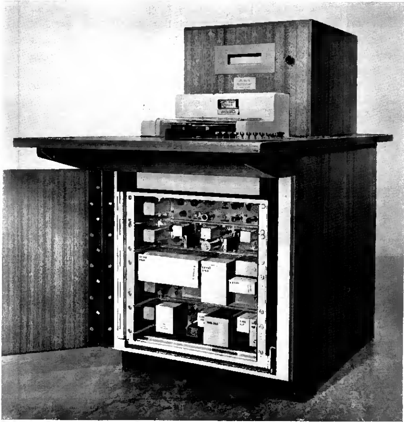
Fig. 8 — Experimental transmitter unit of the bank signature verification system (door open).
