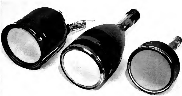
Fig. 20 — Direct-view storage tubes.
