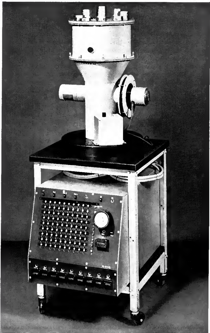
Fig. 2(a) — Open Contact Test Machine (ocrm) is used for exploratory tests of short duration. Single contacts are used instead of twins to increase the failure rate, with usually only one parameter being varied for each test.
