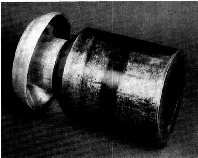
FIG. 26 — Shaving tool partly removed from billet after operation.
